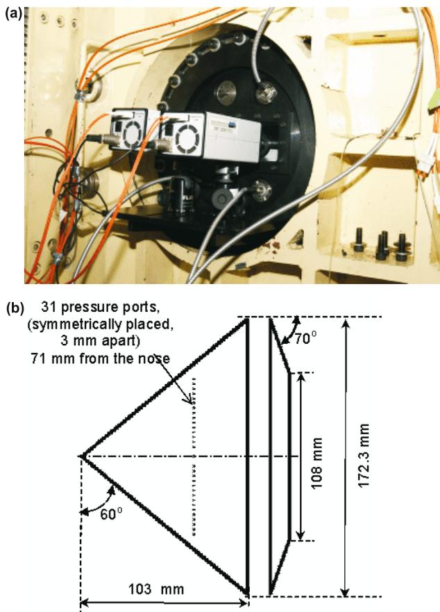
**Figure 2.** PSP arrangement and model details (0.3 trisonic tunnel). (a) PSP system installed on the test-section of 0.3 m trisonic tunnel. (b) Details of the delta-wing model.
