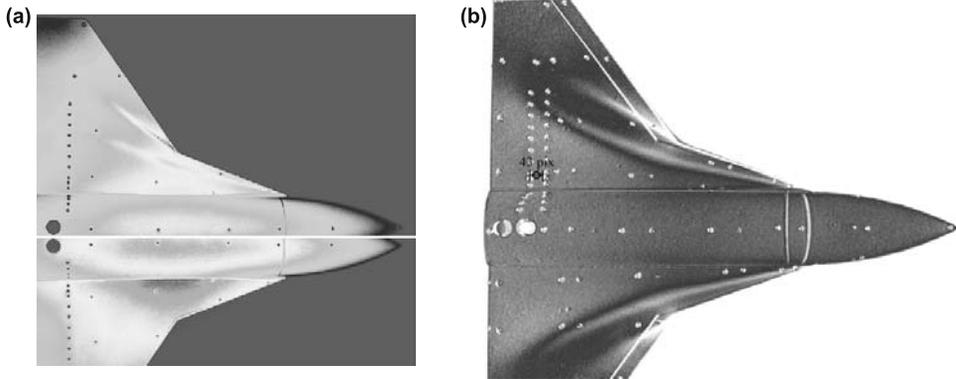
**Figure 3.** Image registration. (a) Image of top-half of the model compared between wind-off and wind-on conditions. (b) Marker misalignment due to camera perspectives.
