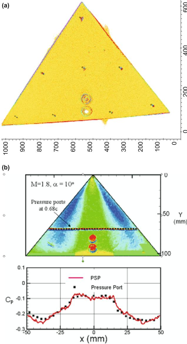
**Figure 6.** Results of the delta-wing model. (a) Skewed field image of the delta-wing model obtained using transformation approach. (b) Pressure map and comparison of PSP data with pressure port data.
