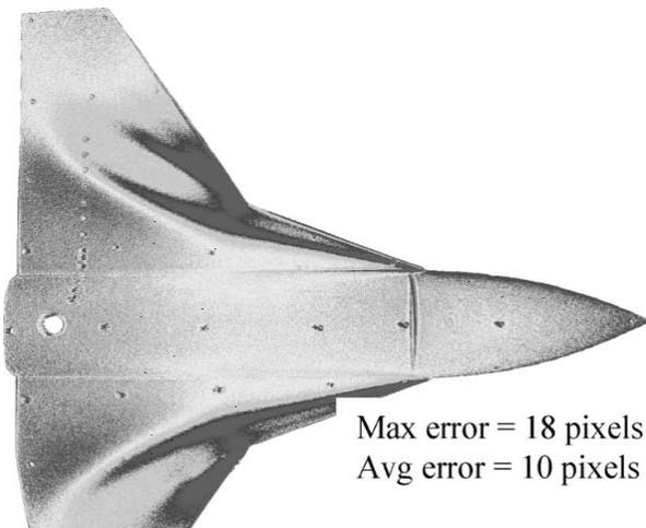
**Figure 4.** Field image using image-warping approach showing maximum and average errors in alignment.
