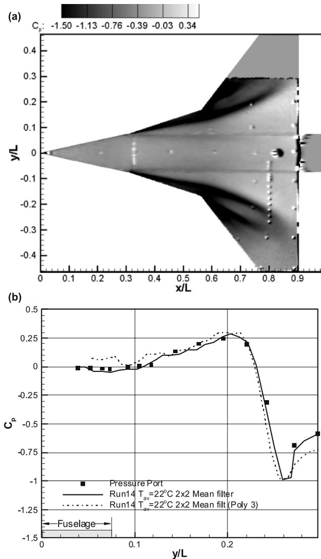
**Figure 5.** Results of the aircraft wing-body model. (a)  $C_p$  on surface grid using resection-before-ratio approach. (b) Comparison of mean pressure at a section from PSP methods and pressure ports.
