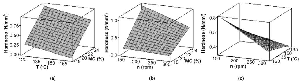
**Figure 6.** (a) Influence of  $T$  and  $MC$  on hardness of extrudate at screw speed 225 rpm. (b) Influence of  $n$  and  $MC$  on hardness of extrudate at temperature 145°C. (c) Influence of  $n$  and  $T$  on hardness of extrudate at moisture content 21.4%. For abbreviations see table 1.
