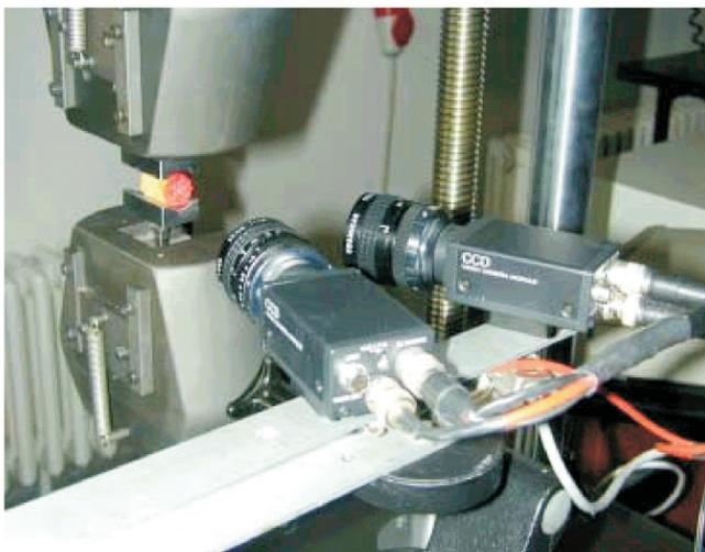
Figure 2. Universal testing machine Messphysik Beta 50–5.
