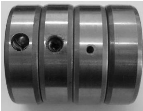
Figure 3. Three bearings with holes drilled through the outer race and an intact bearing.
