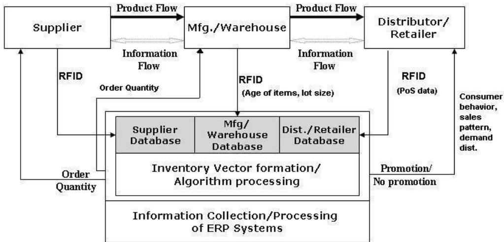
**Figure 3.** An RFID-based architecture for management of perishable inventory.
