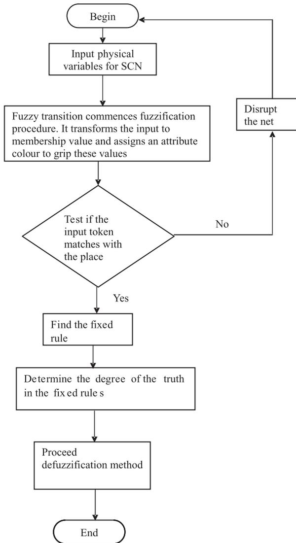
**Figure 7.** Flowchart for FEHLPN algorithm.
