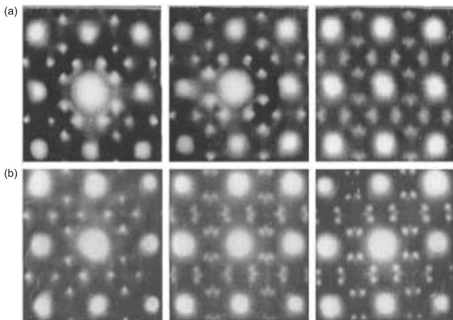
**Figure 3.** Sequence of diffraction patterns showing gradual changes in the Ni-20 at% Mo alloy from the SRO to the LRO state. (a) 573 K and (b) 773 K. The duration and the temperature of irradiation at a dose rate of  $5 \times 10^{-3}$  dpa/s are indicated.  $t_o$  represents the time ( $\sim 5s$ ) elapsed for taking the first exposure.
