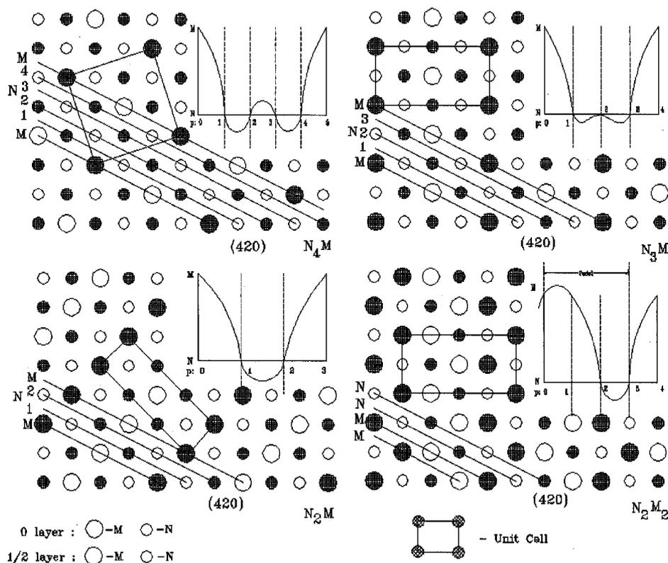
**Figure 1.** Sequences of Ni layers (N) and Mo layers (4 2 0) planes in (a)  $\text{Ni}_4\text{Mo}(D1_a)$ , (b)  $\text{Ni}_3\text{V}(DO_{22})$ , (c) metastable  $\text{Ni}_2\text{Mo}$  and (d)  $\text{N}_2\text{M}_2$  structures. Lattice correspondence between the parent *fcc* and the coherent ordered structures are also shown by marking the vectors  $a_i$  and  $A_i$  corresponding to the unit cells of the former and the latter respectively.
