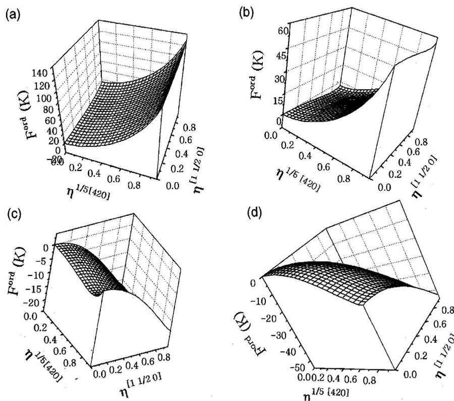
**Figure 6.** The ordering free energy of the  $\text{Ni}_4\text{Mo}$ -based alloy, exhibiting the  $\langle 1\ 1/2\ 0 \rangle$  and  $(1/2)\langle 4\ 2\ 0 \rangle$  ordering tendencies, plotted as a function of order parameters for the corresponding ordering wave vector at four different temperatures, (a) to (d) in decreasing temperature sequence.
