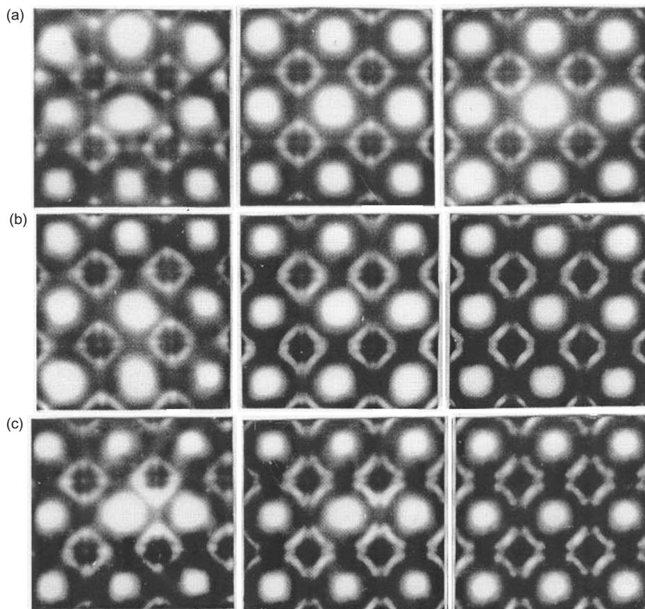
**Figure 4.** Sequence of diffraction patterns  $[0\ 0\ 1]$  zone axis showing the progressive changes in the diffuse intensity distribution as the Ni-25 at% Mo alloy undergoes radiation-induced ordering at different temperatures: (a) 495, (b) 695, and (c) 745 K.
