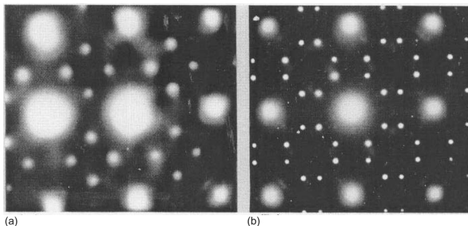
**Figure 2.** [0 0 1] diffraction pattern from stoichiometric Ni<sub>4</sub>Mo alloy: (a) SRO; (b) LRO
