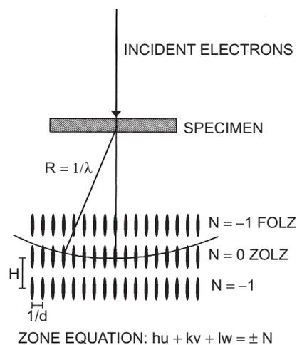
**Figure 4.** Plan view of Ewald sphere construction for electron diffraction.  $R$  represents the radius of the Ewald sphere,  $\lambda$  is the wavelength of incident electrons,  $d$  is the interlunar distance,  $H$  is the reciprocal lattice layer distance, and ZOLZ, FOLZ, SOLZ refer to the zero, first and second order lauer zones respectively. The zone equation is the basis for this classification.
