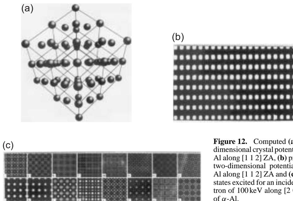
**Figure 12.** Computed (a) three-dimensional crystal potential in  $\alpha$ -Al along  $[1\ 1\ 2]$  ZA, (b) projected two-dimensional potential in  $\alpha$ -Al along  $[1\ 1\ 2]$  ZA and (c) Bloch states excited for an incident electron of 100 keV along  $[2\ 0\ 0]$  ZA of  $\alpha$ -Al.
