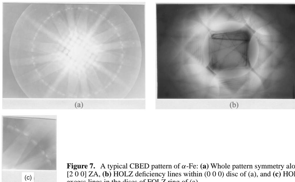
**Figure 7.** A typical CBED pattern of  $\alpha$ -Fe: (a) Whole pattern symmetry along  $[2\ 0\ 0]$  ZA, (b) HOLZ deficiency lines within  $(0\ 0\ 0)$  disc of (a), and (c) HOLZ excess lines in the discs of FOLZ ring of (a).
