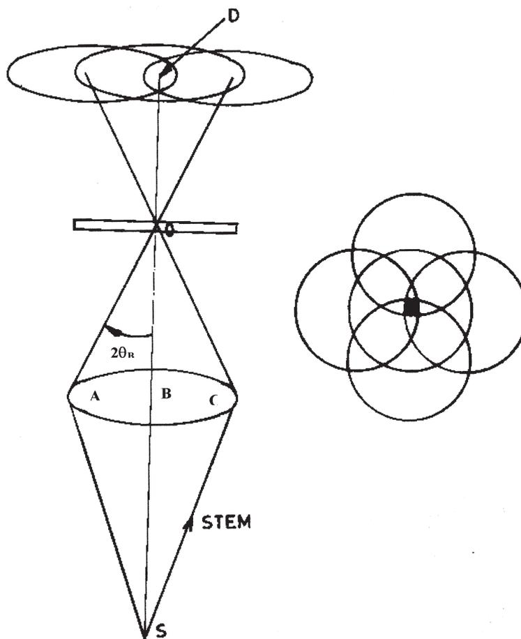
**Figure 16.** Axial three-beam lattice imaging in STEM, with an illumination angle twice the Bragg angle. Three orders overlap at *D*. The appearance of a two-dimensional coherent CBED pattern used for axial five beam imaging is shown at the right.
