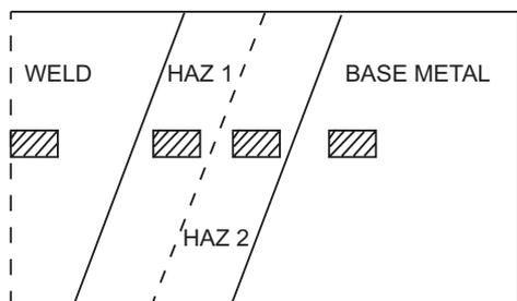
**Figure 8.** Schematic representation of the regions selected for study of variation of lattice strain by CBED experiments.
