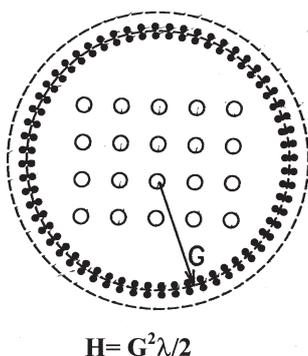
**Figure 5.** Sectional view of Ewald sphere showing radius of the FOLZ ring –  $G$ .  $H$  – reciprocal lattice layer distance, is related to  $G$  and  $\lambda$ .
