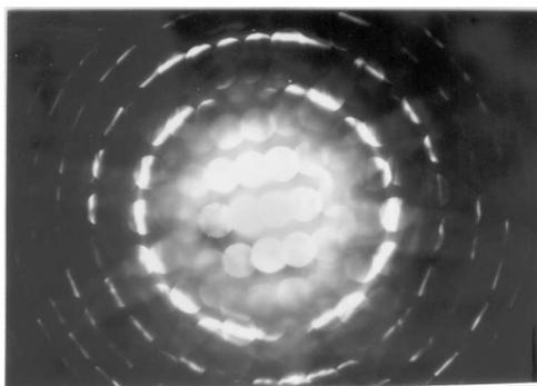
**Figure 6.** A typical CBED pattern along  $[0\ 6\ \bar{6}]$  ZA of  $\text{Al}_6\text{Mn}$  showing HOLZ rings to derive three-dimensional information about the reciprocal lattice ( $ZA = \text{zone axis}$ ).
