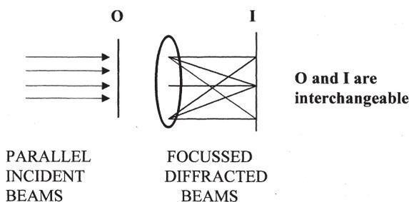
**Figure 3.** Reciprocity theorem illustrating the interchangeability of the incident and diffracted beams.
