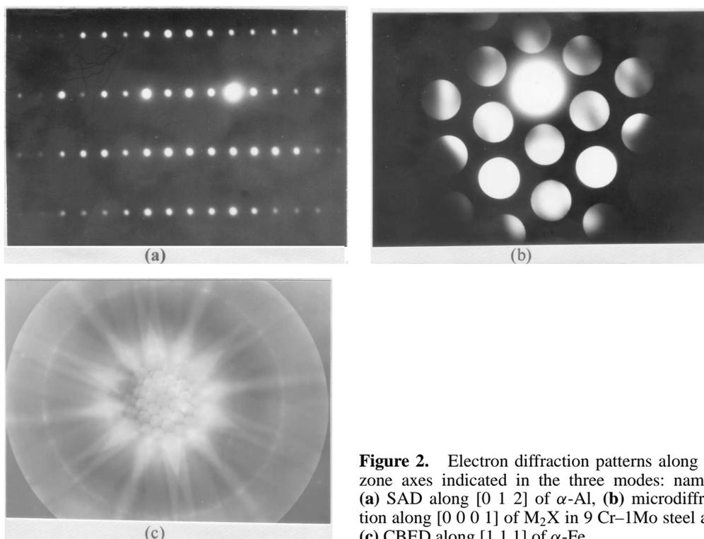
**Figure 2.** Electron diffraction patterns along the zone axes indicated in the three modes: namely (a) SAD along  $[0\ 1\ 2]$  of  $\alpha$ -Al, (b) microdiffraction along  $[0\ 0\ 0\ 1]$  of  $M_2X$  in 9 Cr-1Mo steel and (c) CBED along  $[1\ 1\ 1]$  of  $\alpha$ -Fe.
