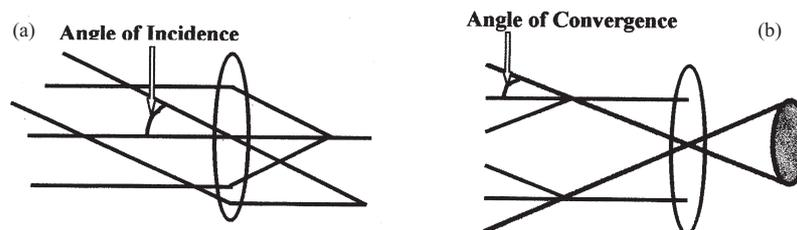
**Figure 1.** Electron diffraction in two different geometries. (a) Selected area diffraction (SAD) and (b) convergent beam electron diffraction (CBED).
