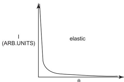
**Figure 10.** Angular distribution of the intensity of elastically, scattered electrons.
