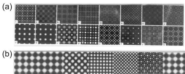
**Figure 15.** Smearing of Bloch states excited along  $[2\ 0\ 0]$  ZA in  $\alpha$ -Al, for an incident electron of 100 keV, with increase in DW factor: (a)  $0.005$  and (b)  $0.3\ \text{nm}^{-1}$ .
