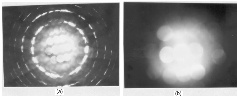
**Figure 13.** Reduction in the number of HOLZ rings in CBED patterns of  $\text{Al}_6\text{Mn}$  due to ion irradiation (100 keV argon ion): (a) unirradiated and (b)  $2 \times 10^{14}$  ions/cm<sup>2</sup>.
