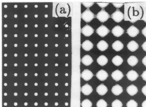
**Figure 14.** Smearing of projected potential along [2 0 0] ZA in  $\alpha$ -Al, with increase in Debye Waller factor: (a) 0.005 and (b) 0.3 nm<sup>-1</sup>.
