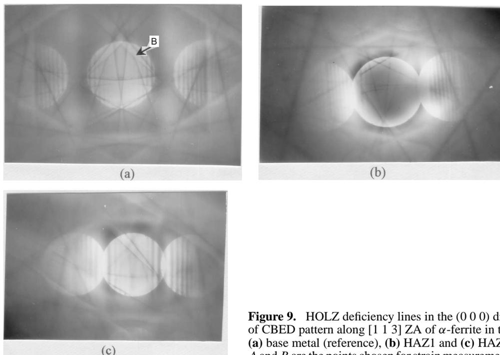
**Figure 9.** HOLZ deficiency lines in the (0 0 0) disc of CBED pattern along [1 1 3] ZA of  $\alpha$ -ferrite in the (a) base metal (reference), (b) HAZ1 and (c) HAZ2. A and B are the points chosen for strain measurement.
