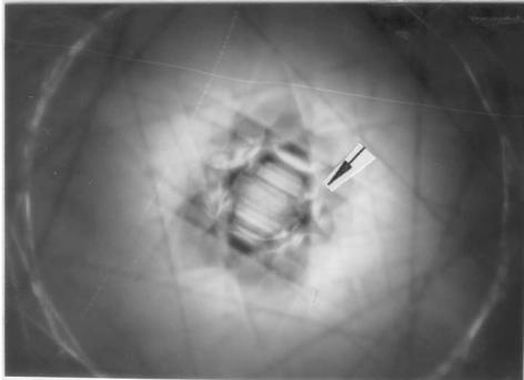
**Figure 11.** CBED pattern of  $\alpha$ -ferrite along  $[1\ 1\ 3]$  ZA showing the interference pattern near the Brillouin zone boundary (arrow marked).
