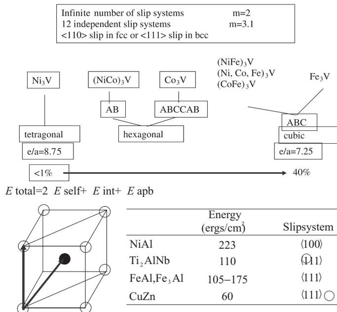
**Figure 4.** The influence of crystal structure and APB energy on the operative slip system.
