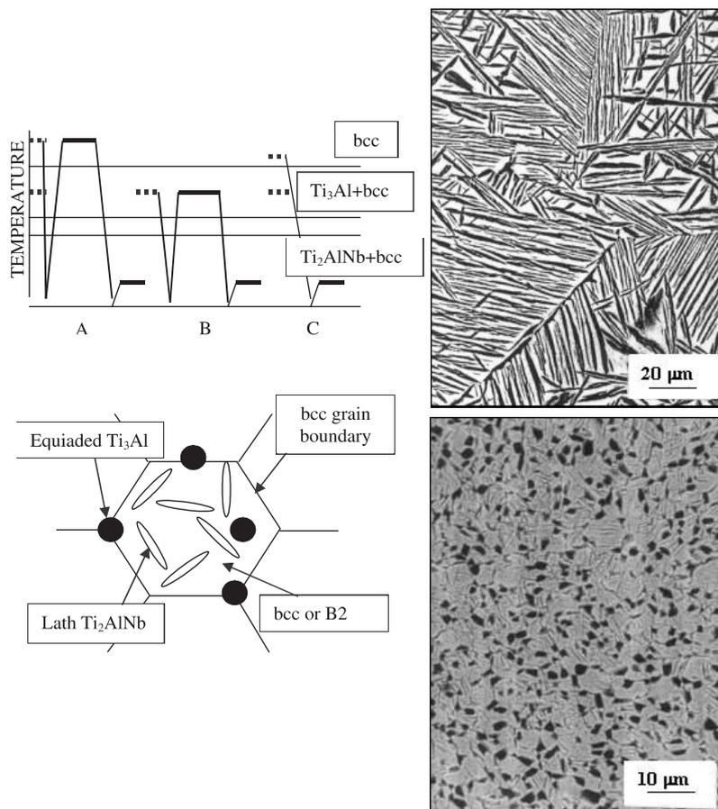
**Figure 11.** Processing sequences in  $Ti_2AlNb$  base alloys along with a schematic description of various microstructural parameters. The dashed lines indicate hot working sequences. Two typical microstructural variants are also shown.
