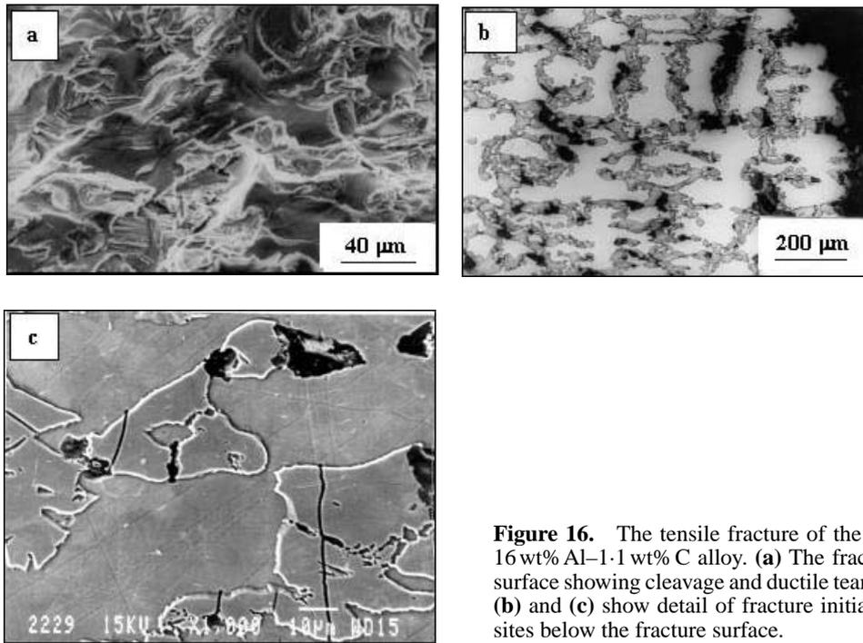
**Figure 16.** The tensile fracture of the Fe–16 wt% Al–1.1 wt% C alloy. (a) The fracture surface showing cleavage and ductile tearing; (b) and (c) show detail of fracture initiation sites below the fracture surface.
