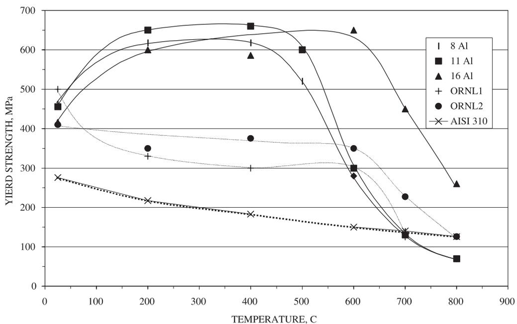
**Figure 17.** Yield stress of the Fe<sub>3</sub>Al–C alloys containing 1.1 wt% C as a function of temperature in relation to stainless steel, and vacuum melted and wrought Fe<sub>3</sub>Al base alloys developed at ORNL, USA.
