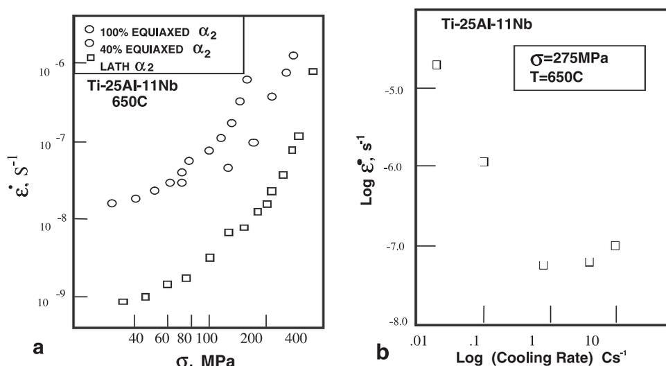
**Figure 9.** The creep of  $Ti_3Al$ –Nb phase alloys; (a) the effect of equiaxed  $Ti_3Al$  volume fraction on steady state creep; (b) the effect of cooling rate after solution treatment in the *bcc* phase region on steady state creep (Banerjee *et al* 1993).
