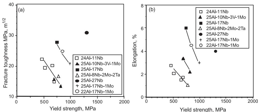
**Figure 5.** The evolution of strength, ductility and toughness with increasing Nb content in Ti<sub>3</sub>Al–Nb and Ti<sub>2</sub>AlNb alloys. (a) Fracture toughness as a function of yield strength in alloys of different Nb content (b) Elongation as a function of yield strength in alloys of different Nb content (Banerjee 1994).
