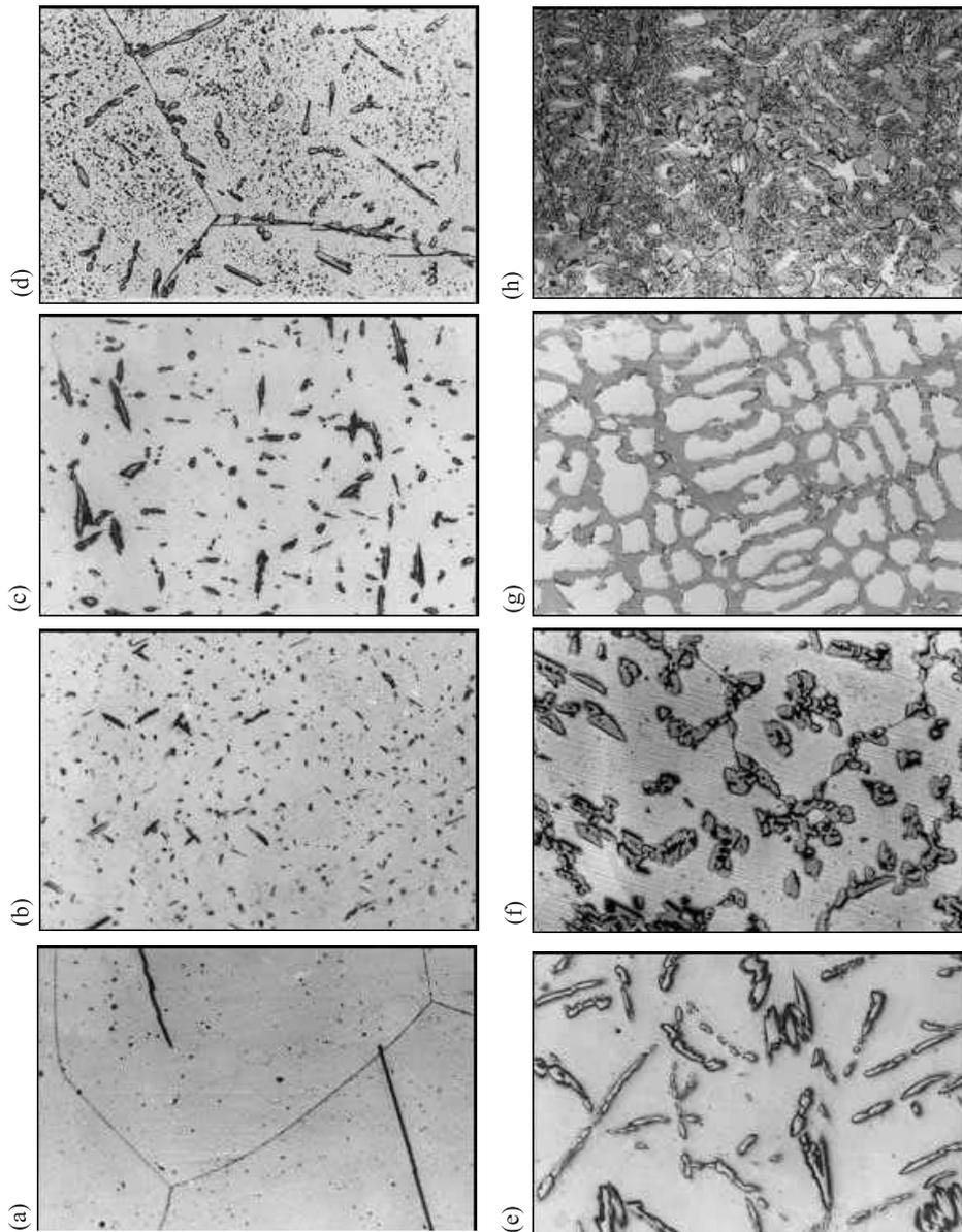
**Figure 14.** The effect of C content on as-cast microstructures of Fe-16 wt.% Al alloys as a function of carbon content; **(a)** 0.03 wt.% C, **(b)** 0.07 wt.% C, **(c)** 0.14 wt.% C, **(d)** 0.27 wt.% C, **(e)** 0.5 wt.% C, **(f)** 1.1 wt.% C, **(g)** 1.8 wt.% C, **(h)** 1.8 wt.% C.
