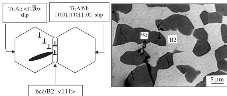
**Figure 7.** A schematic illustration of crack initiation and blunting, along with operative slip systems in *bcc* /B2,  $Ti_3Al$ , and  $Ti_2AlNb$  base alloys. The micrograph shows cleavage cracks in  $Ti_3Al$  blunted at the B2 phase.
