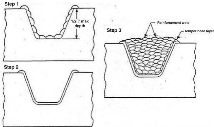
**Figure 1.** Temper-bead weld repair and weld temper-bead reinforcement by the SMAW process. (Step 1: Butter cavity with one layer of weld metal with a 2.5 mm diameter coated electrode. Step 2: Remove the weld crown of the first layer by grinding or machining. Step 3: The second layer is deposited with a 3.15 mm diameter electrode, and the subsequent layers with welding electrodes no larger than 4 mm diameter.)
