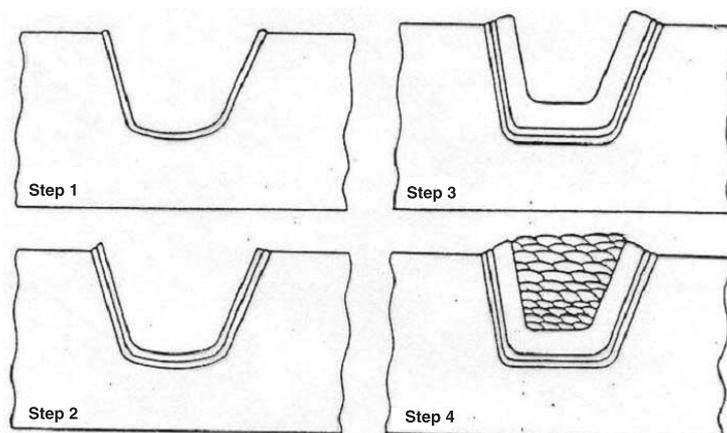
**Figure 2.** Automatic or machine (GTAW) temper-bead weld repair. (Step 1: Deposit layer one with first layer weld parameters used in qualifications. Step 2: Deposit layer two with second layer weld parameters used in qualifications. Step 3: Deposit next four layers with layer three through six weld parameters used in qualifications. Step 4: Subsequent layers to be deposited as qualified.)
