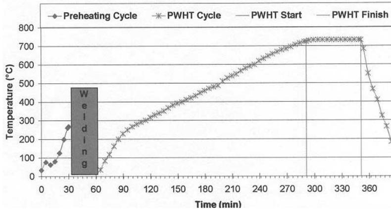
**Figure 9.** Record of time-temperature measurements during preheating at 523 K (250°C) and PWHT at 1008 K (735°C) for 1 h that was used during on-site repair welding of a cracked HP-III shroud using ER410 filler metal.
