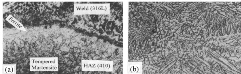
**Figure 14.** *In-situ* metallography microstructures of a repair weldment (made using ER316L filler metal) in the IV-stage of a LP turbine blade after 873 K/1 h PWHT: (a) blade/316L weld interface, and (b) 316L weld metal.
