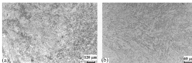
**Figure 15.** Optical photomicrographs of the weld interface region of weldments (made using ER410 filler metal) after 1008 K/1 h PWHT: (a) repair-welded shroud in the III-stage of a HP turbine (by *in-situ* metallography), and (b) procedure qualification weld.
