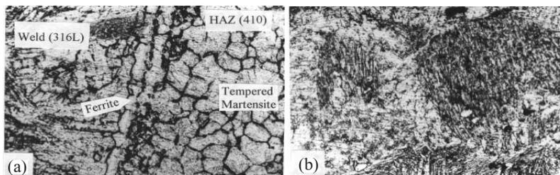
**Figure 13.** In-situ metallography microstructures of a repair weldment (made using ER316L filler metal) in the III-stage of a LP turbine shroud after 873 K/1 h PWHT: (a) shroud/316L weld interface; and (b) 316L weld metal.
