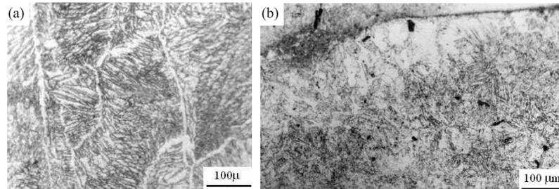
**Figure 16.** In-situ metallography microstructures of repair weldments, made using ER316L filler metal, after service for two years: (a) fusion zone in the IV-stage blade of a LP turbine, and (b) HAZ near fusion line in the III-stage shroud of a HP turbine.
