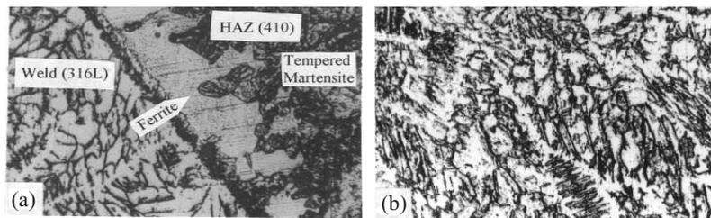
**Figure 12.** In-situ metallography microstructures of a mock-up weldment (made using ER316L filler metal) after 873 K/1 h PWHT: (a) 410 SS/316L weld interface, and (b) 316L weld metal.
