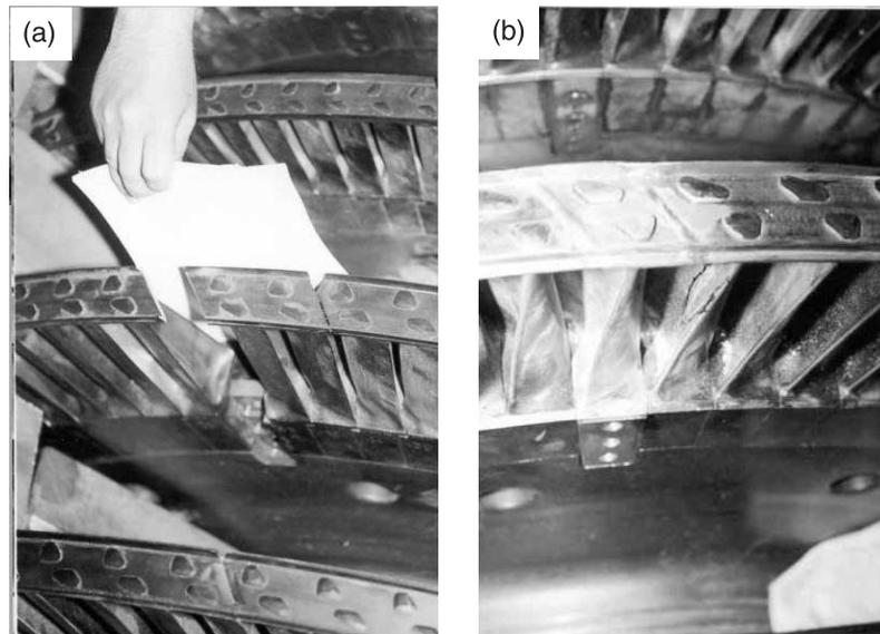
**Figure 11.** Photographs of the III-stage of a HP turbine showing the shroud: (a) after cutting and removal of the root-cracked blade, and (b) after *in-situ* re-welding using E316L filler metal subsequent to blade replacement.
