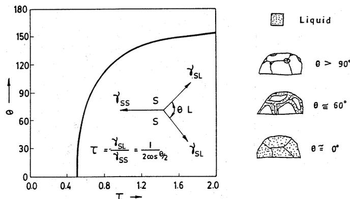
**Figure 6.** The variation of dihedral contact angle between liquid and solid phases with surface energy ratio; the change in grain wetting behaviour with decreasing wetting angle is also illustrated.
