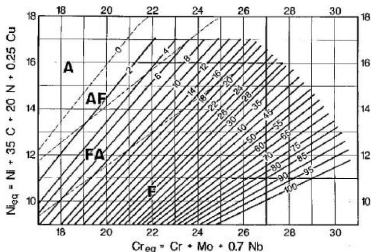
**Figure 4.** The WRC-92 constitution diagram for weld metal ferrite, including solidification mode boundaries.
