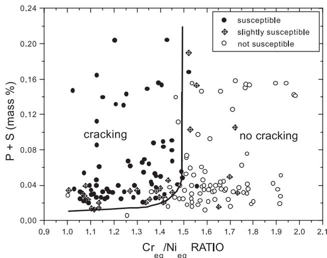
**Figure 8.** Solidification cracking behaviour in austenitic stainless steel welds as a function of Schaeffler  $Cr_{eq}/Ni_{eq}$  ratio and P+S levels (after Kujanpaa *et al* 1979).
