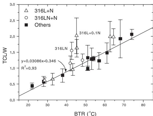
**Figure 14.** Correlation between TCL in longitudinal varestraint test and BTR ( $R^2$  is the correlation coefficient and the equation shown is an error-weighted fit).
