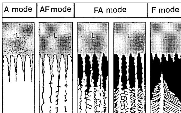
**Figure 3.** Schematic representation of solidification modes in austenitic stainless steel welds showing phase morphologies (after Koseki & Flemings 1996).
