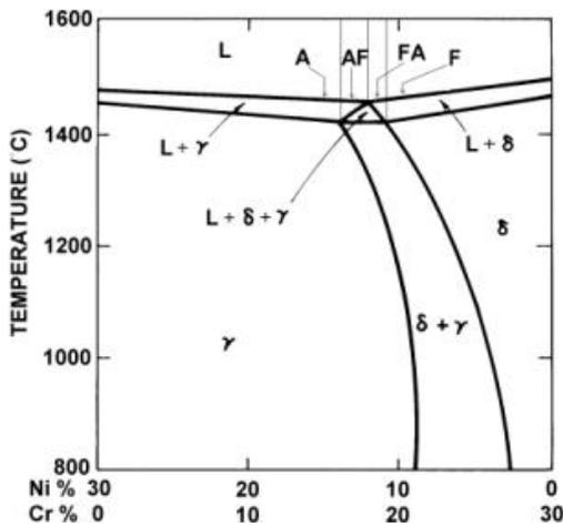
**Figure 2.** Pseudobinary section of the Fe–Cr–Ni ternary diagram at 70% Fe, showing solidification modes; A - fully austenitic, AF - austenitic–ferritic, FA - ferritic–austenitic and F - fully ferritic.
