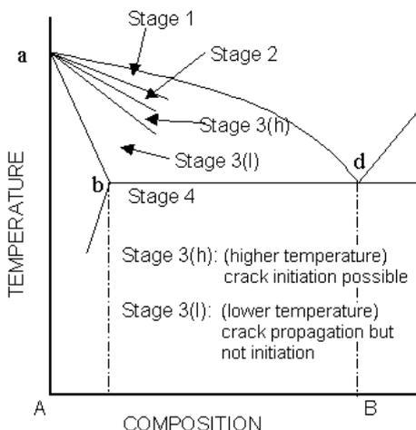
**Figure 7.** Modified concept of the effect of constitution on cracking susceptibility in binary systems (Matsuda 1990).
