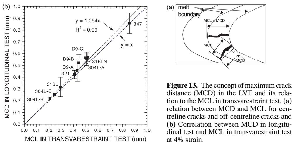
**Figure 13.** The concept of maximum crack distance (MCD) in the LVT and its relation to the MCL in transvarestraint test, (a) relation between MCD and MCL for centreline cracks and off-centreline cracks and (b) Correlation between MCD in longitudinal test and MCL in transvarestraint test at 4% strain.
