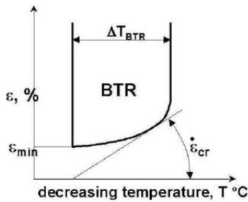
**Figure 12.** The concept of brittleness temperature range (BTR) during solidification of metals in the strain-temperature regime (after Prokhorov & Prokhorov 1971).
