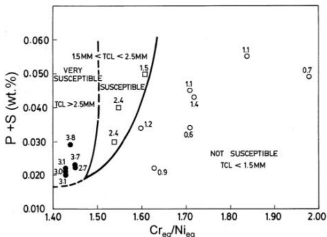
**Figure 9.** Solidification cracking behaviour in austenitic stainless steel welds as a function of Hammar–Svensson  $Cr_{eq}/Ni_{eq}$  ratio and P+S levels (Lundin *et al* 1988).
