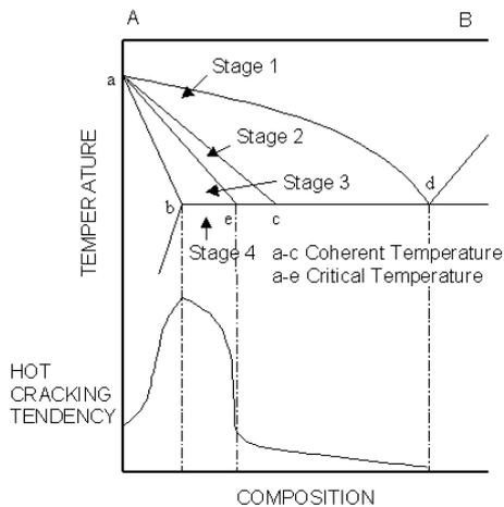
**Figure 5.** Effect of constitutional features on cracking susceptibility in binary systems according to the generalized theory of Borland (1960).
