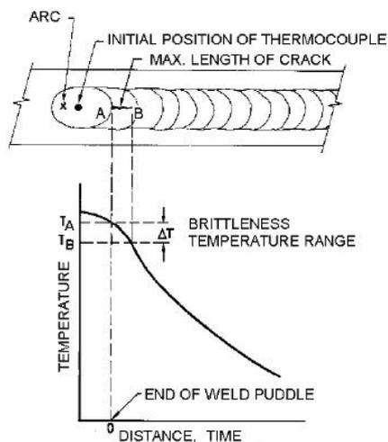
**Figure 11.** Procedure for calculating BTR from the MCL and weld centreline cooling curve (after Lundin & Savage 1965).
