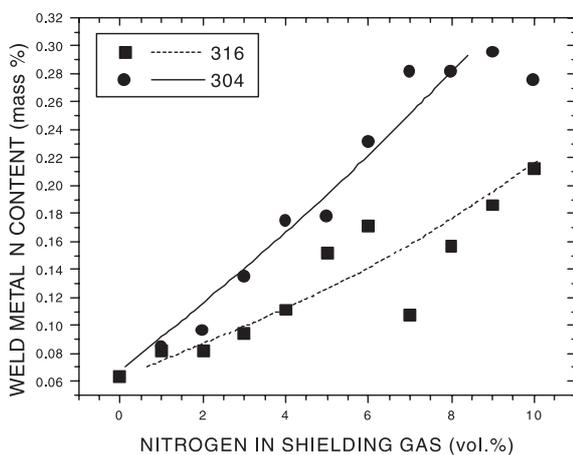
**Figure 10.** Nitrogen content obtained in weld metal as a function of nitrogen content in argon shielding gas for type 304 and 316 weld metals (data of Mudali *et al* 1986).
