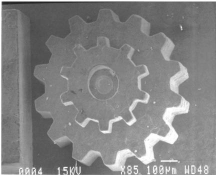
**Figure 2.** Stepped LIGA gear wheels made of 316L stainless steel. Structural height is about  $480\ \mu\text{m}$  and minimum tooth width about  $50\ \mu\text{m}$ ; both values were measured after sintering.
