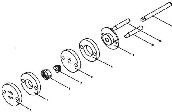
**Figure 4.** Principle drawing of the micro annular gear pump. Outer diameter: 3.2 mm.
