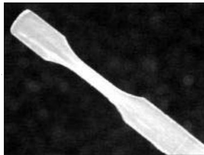
**Figure 8.** Tensile test bars ( $ZrO_2$ , green part) with details in  $\mu m$ .
