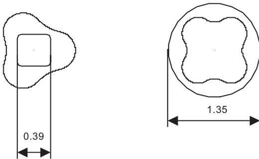
**Figure 5.** Details of the annular gear pump in millimetre.
