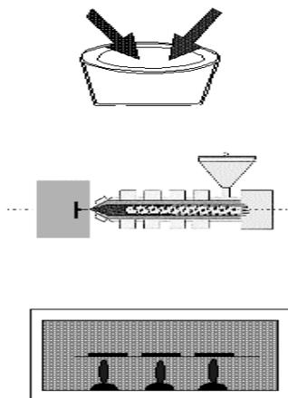
**Figure 1.** Schematic principle of powder injection moulding consisting of three steps: Mixing of feedstock, micro injection moulding, debinding/sintering.
