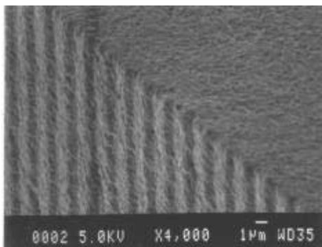
**Figure 3.** Detail of powder injection-moulded micro grid test structure with a zig-zag height of approx.  $0.9\ \mu\text{m}$  in zirconium oxide (bottom).
