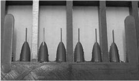
**Figure 7.** Bending bars (17-4PH steel, green parts) for micromechanical tests.
