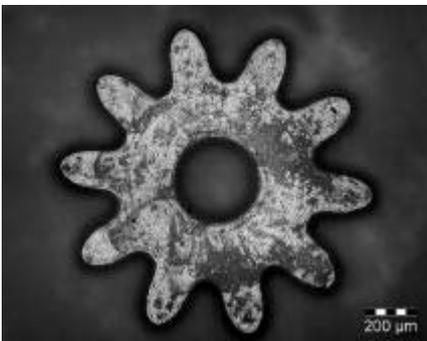
**Figure 9.** Sintered  $ZrO_2$  micro gearwheel, outer diameter 1260  $\mu m$ .
