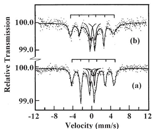
**Figure 2.** Mössbauer spectra for sample with composition 50 Ni<sub>3</sub>Fe–50 SiO<sub>2</sub> and particle size 19.6 nm at (a) room temperature, (b) 77 K (Pal *et al* 2000).
