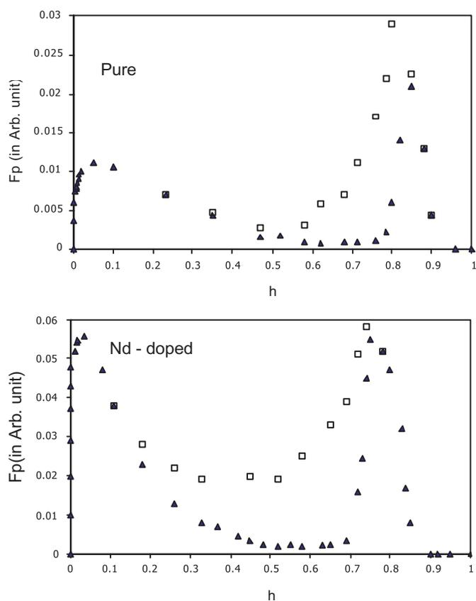
**Figure 3.** Measured pinning force vs. field (in reduced units,  $h = H/H_{C2}$ ) for two samples of  $\text{CeRu}_2$ . The squares correspond to measurements in the field-cooled (FC) state, while the triangles correspond to the zero-field-cooled (ZFC) state. In the region below the peak effect, the pinning is stronger in the FC state.
