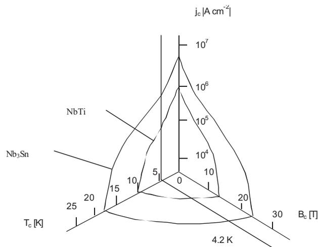
**Figure 2.** The operating volume of a superconducting material, where it has zero resistivity, is enclosed by the  $T_C$ ,  $H_{C2}$  and  $J_C$  lines. The figure shows these lines for NbTi and Nb<sub>3</sub>Sn, the two superconducting materials in commercial use.
