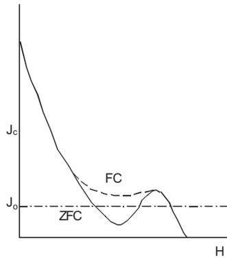
**Figure 4.** Schematic of the history-dependence in  $J_C$  vs. field  $J_C$  is higher in the FC state. If the measuring current used is  $J_0$  as indicated, then a finite resistance is seen in the ZFC state at intermediate fields, whereas no resistance is seen in the FC state (Chaudhary *et al* 2001).
