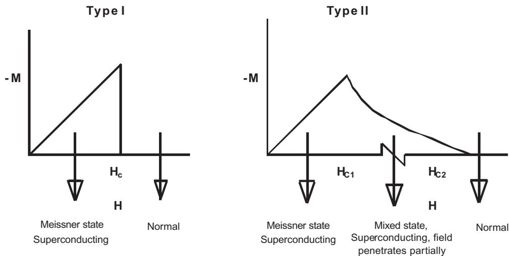
**Figure 1.** The schematic magnetisation behaviour of type I and type II superconductors is shown. In the Meissner state they behave as perfect diamagnets, and so magnetic flux penetrates the bulk of the sample. The mixed state of type II superconductors has zero resistivity but allows partial flux penetration, in the form of quantised vortices.
