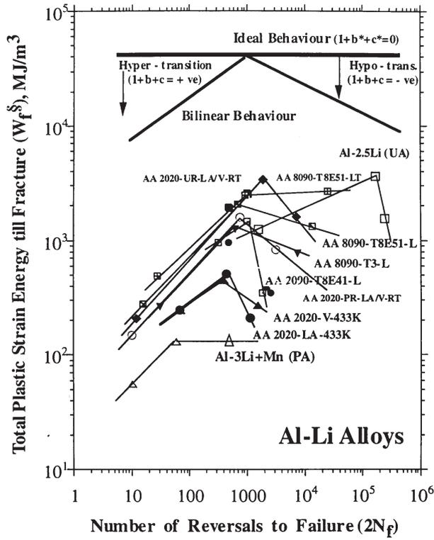
**Figure 10.** Variation of total cyclic plastic strain energy till fracture  $W_f^S$  with number of reversals to failure  $2N_f$  for various Al–Li alloys: note that with exception of Al-3wt.%Li + Mn and AA 8090–T8E51 in LT direction, all other alloys exhibit bilinear behaviour shown schematically at the top of figure (from Eswara Prasad & Rama Rao 2000).
