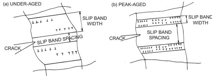
**Figure 14.** Schematic diagram showing the increase in the ratio of slip band spacing to its width, as occurs from the (a) under-aged condition to the peak-aged (b) condition, leading to the increasing extent of co-planar slip with ageing.
