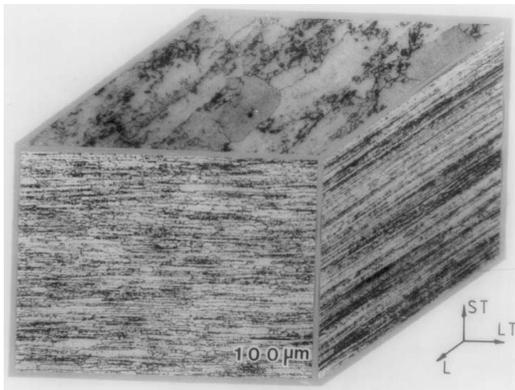
**Figure 1.** Triplanar optical micrograph of a commercial (Alcan) Al–Li alloy AA 8090 in T8E51 condition, showing wide variation in grain width and aspect ratio in the three orthogonal directions (from Eswara Prasad 1993).
