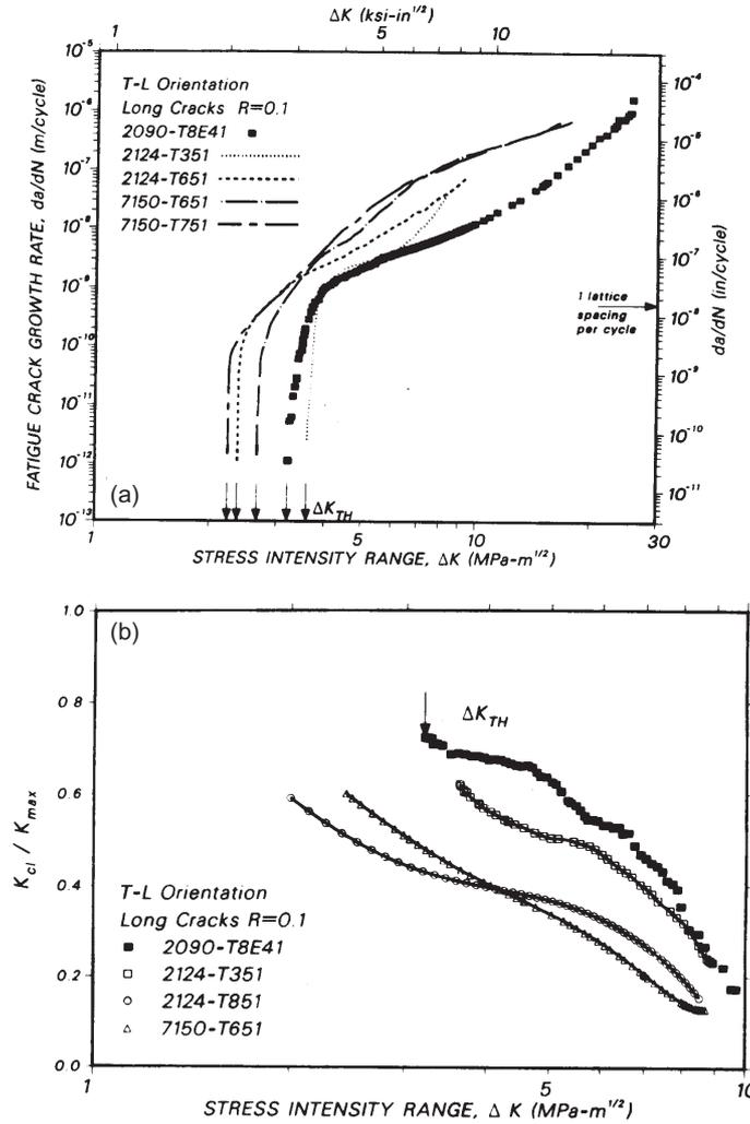
**Figure 16.** Fatigue crack growth behaviour of several Al alloys as compared to the Al–Li alloy AA2090–T8E41: (a) variation of crack growth rates and (b) extent of crack closure ( $K_{cl}/K_{max}$ ) with  $\Delta K$ . The AA 2090 alloy exhibits superior FCG resistance due to higher extent of crack closure (Venkateswara Rao *et al* 1991).
