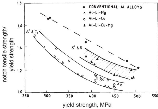
**Figure 12.** Variation in the ratio of NTS and yield strength (YS) of Al-Li alloys strengthened with  $\delta'$  and  $T_1$  (in Al-Li with Mg or Cu) and  $\delta'$  and S (Al-Li with both Mg and Cu). Note the enhancement in the toughness (the ratio of NTS/YS) that occurs from S' precipitates as a result of simultaneous addition of Mg and Cu (from Gregson 1984).
