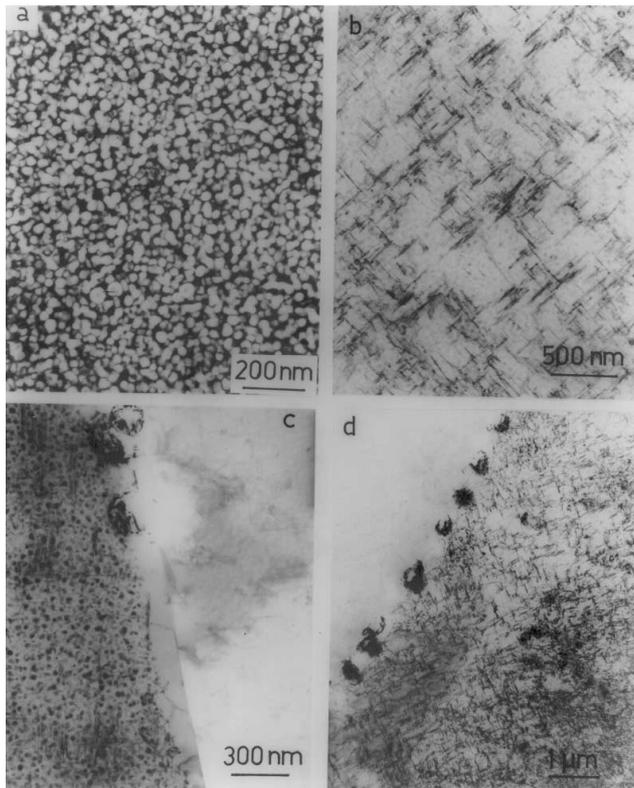
**Figure 3.** Transmission electron micrographs of AA 8090-T8E51 alloy plate showing (a) distribution of  $\delta'$  precipitates, (b) distribution of  $S$  precipitates, (c)  $\delta'$ -precipitate free zones, and (d) network of  $T_2$  ( $\text{Al}_6\text{CuLi}_3$ ) precipitates along the high angle grain boundary.
