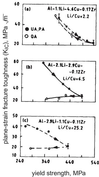
**Figure 13.** Variation of plane-strain fracture toughness ( $K_{Ic}$ ) with yield strength in case of Al-Li-Cu alloys with varied Li and Cu contents: (a) Li/Cu = 2.2 (ratio of atomic %), (b) Li/Cu = 6.5 and (c) Li/Cu = 25.2 (from Suresh *et al* 1987).
