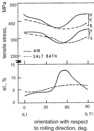
**Figure 7.** Variation in tensile properties with respect to the rolling direction. The alloy, heat treated using salt bath shows higher degree of isotropy, especially tensile elongation (from Reynolds *et al* 1986).
