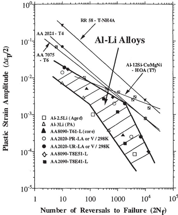
**Figure 9.** Comparison of LCF resistance of Al-Li alloys with that of traditionally used aircraft structural Al alloys, based on plastic strain amplitude ( $\Delta\epsilon_p/2$ ) (from Eswara Prasad & Rama Rao 2000).
