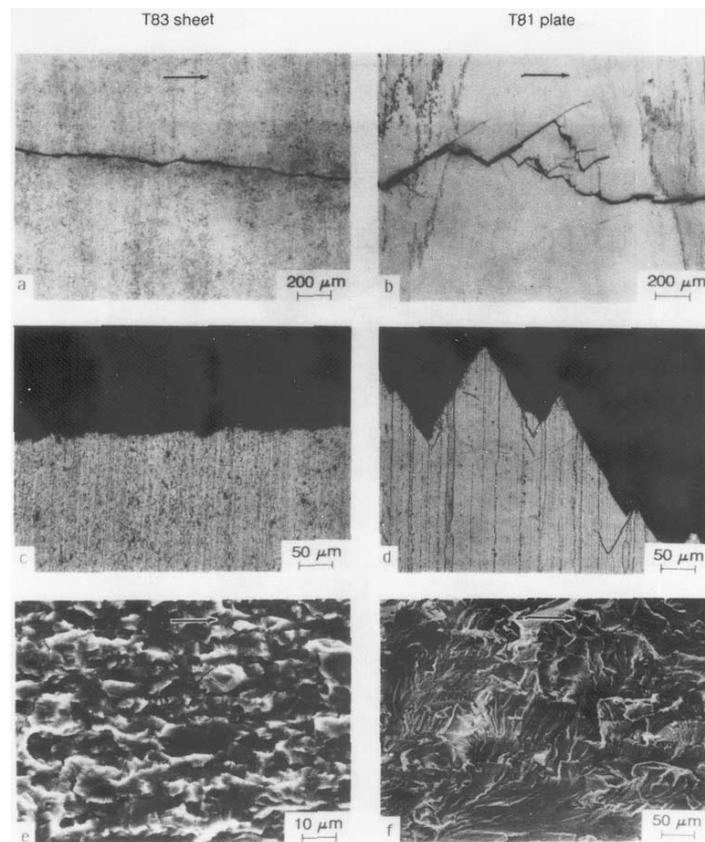
**Figure 18.** Comparison of fatigue crack path and fracture surface morphologies in AA 2090 alloy processed as T83 sheet and T81 plate, showing (a, b) crack paths along the crack growth direction, (c, d) crack profiles across the specimen thickness and (e, f) fracture surfaces. Arrows indicate the general direction of crack growth (from Venkateswara Rao *et al* 1991).
