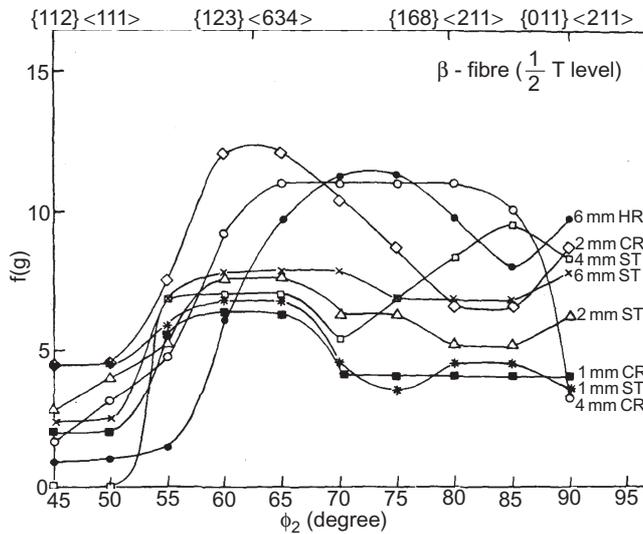
**Figure 4.** Intensities of various texture components at half thickness level for an AA 8090 alloy processed to various stages by hot rolling (HR), cold rolling (CR) and solution treatment (ST). Major texture components such as copper  $\{112\}\langle 111\rangle$ , S  $\{123\}\langle 634\rangle$ , brass S  $\{168\}\langle 211\rangle$  and brass  $\{011\}\langle 211\rangle$  have been indicated.
