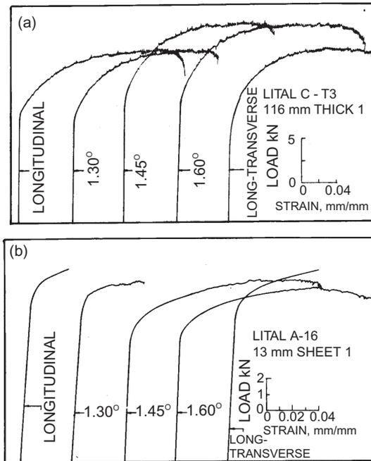
**Figure 5.** Load–strain plots of AA 8090 Al–Li alloys in (a) underaged (Lital C-T3) and (b) peakaged (Lital A-T6) conditions. Except for L and LT directions in the peak-aged alloy, in the other conditions the alloys exhibit serrated yielding and co-planar slip (from Eswara Prasad & Malakondaiah 1992).
