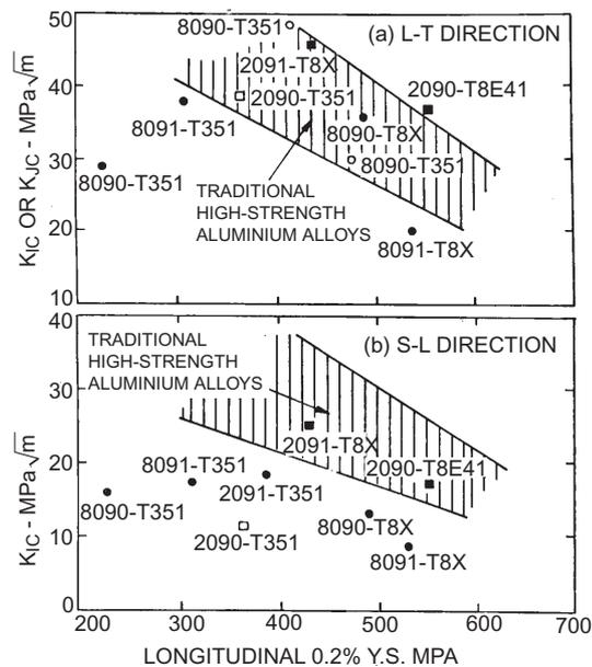
**Figure 15.** Fracture resistance of Al–Li alloys in L–T (notch being oriented perpendicular to the rolling direction) and S–L (notch being oriented in the through-thickness direction) notch orientations (from Venkateswara Rao & Ritchie 1989).
