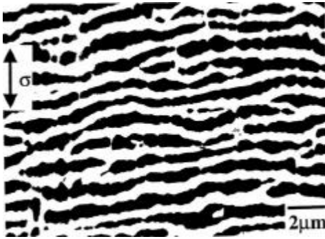
Figure 2. SEM micrograph showing rafting in SX superalloy.
