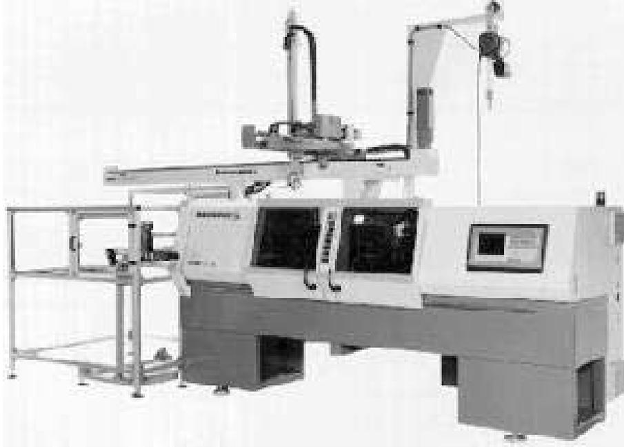
**Figure 4.** Powder injection moulding machine.
