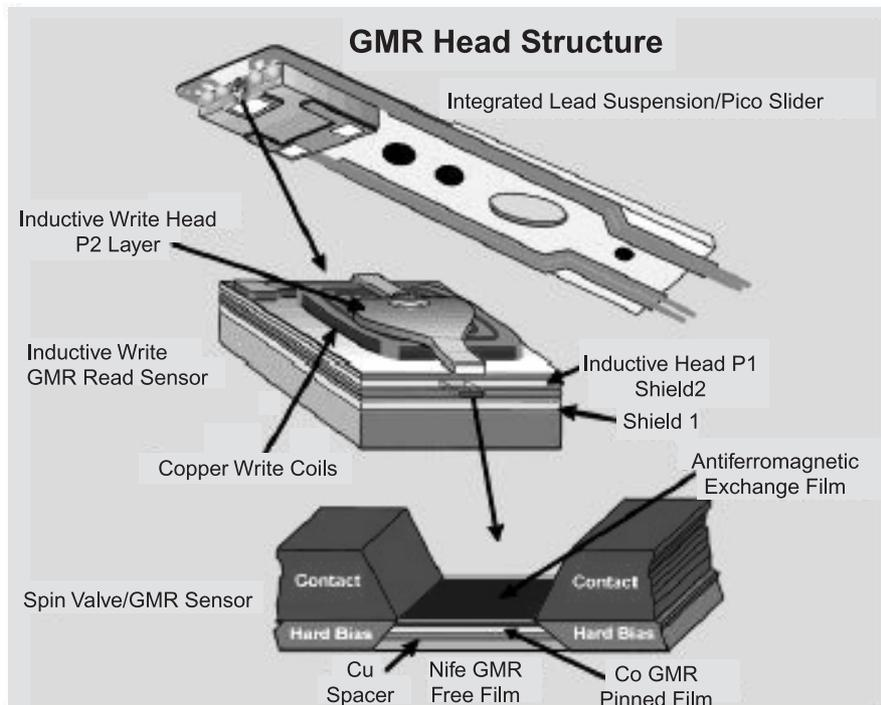
**Figure 1.** IBM commercial GMR read head.
