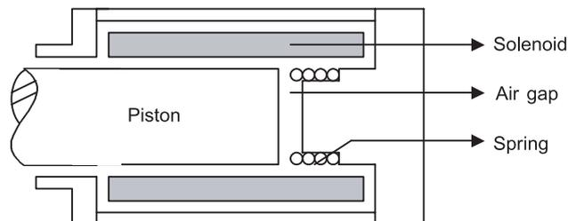
**Figure 6.** Schematic of a solenoid unit.
