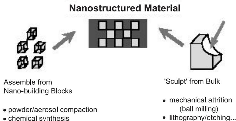
**Figure 2.** Ways to make nanostructured material.
