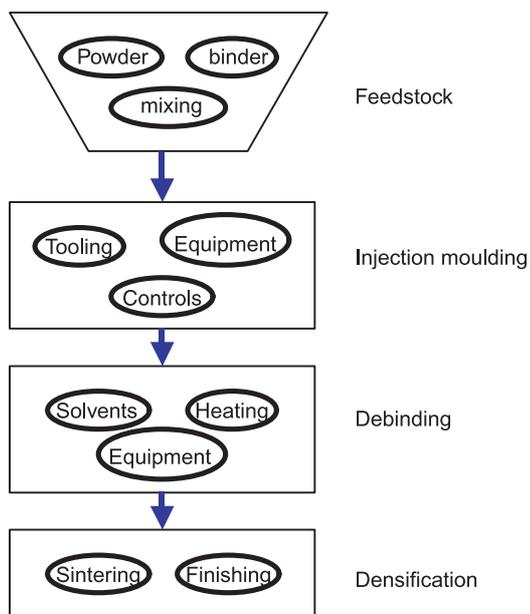
**Figure 3.** Flow chart for the PIM process showing the four major process steps.
