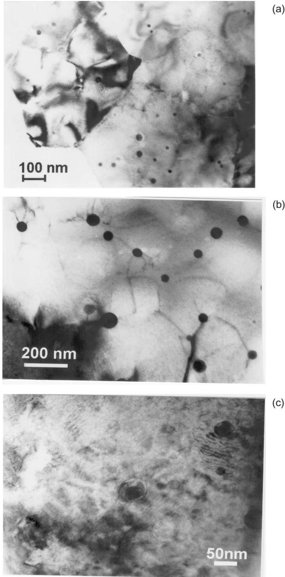
**Figure 5.** Bright field micrographs of bismuth particles embedded in Al-Cu-Fe matrix. **(a)** As melt-spun sample. Strain in the matrix is evident. **(b)** Annealed at 800°C. Low angle boundaries and dislocations are observed in the matrix. **(c)** Annealed at 600°C. The matrix is microcrystalline.
