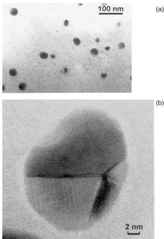
**Figure 1.** (a) A bright field micrograph showing the distribution of Pb particles in as melt-spun Al<sub>75</sub>Cu<sub>15</sub>V<sub>10</sub> alloy (amorphous matrix). (b) A high resolution image of a Pb particle in icosahedral matrix. The particle is multiply twinned. Some facets with the matrix are observed.
