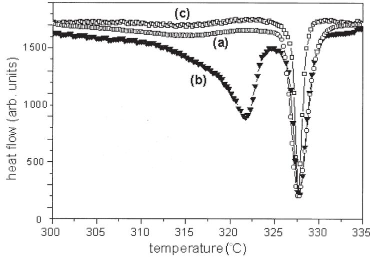
**Figure 4.** Parts of DSC traces showing melting of lead particles in Al–Cu–Fe matrix in (a) the as melt-spun condition, (b) annealed at 800°C and (c) at 600°C.
