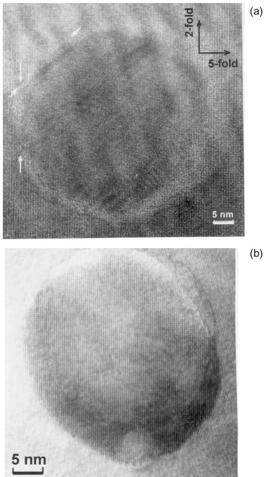
**Figure 6.** Lattice images of bismuth particles in Al-Cu-Fe matrix. **(a)** Annealed at 800°C. fivefold and twofold planes perpendicular to each other are observed in this zone axis of the matrix. Faceting is observed on the particle (for example, on twofold planes on the left side of the micrograph, marked by arrows). **(b)** In sample annealed at 600°C. No faceting or coherence with the matrix is evident.
