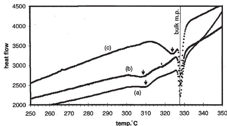
**Figure 2.** Part of DSC traces for heating runs on the Al–Cu–V samples showing melting of lead in (a) amorphous matrix, (b) a mixture of amorphous and quasicrystalline matrix and (c) quasicrystalline matrix.
