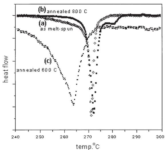
**Figure 7.** Parts of DSC traces showing the melting of bismuth particles in Al-Cu-Fe matrix in **(a)** as melt-spun sample, **(b)** sample annealed at 800°C and **(c)** at 600°C.
