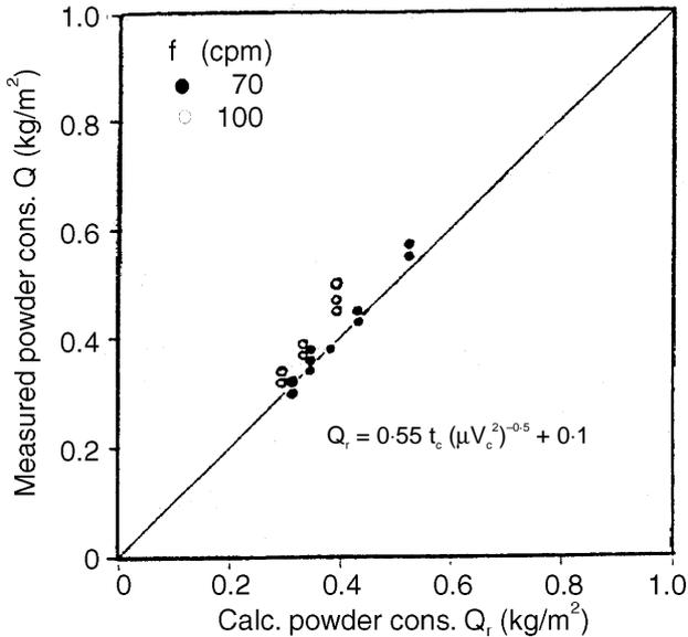
**Figure 10.** Comparison of measured and calculated powder consumption (Wolf 1991a).
