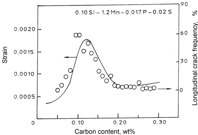
**Figure 16.** Correspondence of calculated strain with frequency of longitudinal crack formation (Kim *et al* 1996).
