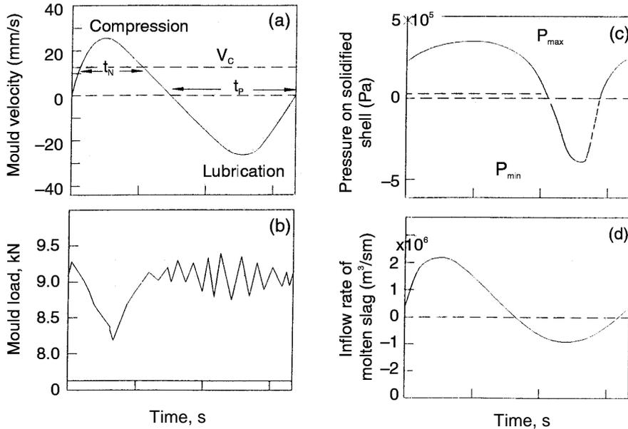
**Figure 1.** Effect of mould oscillation on (a) negative and positive strip time ( $t_n$ ,  $t_p$ ), (b) mould load representing friction (Brendzy *et al* 1993), (c) slag pressure on solidified shell (Takeuchi *et al* 1991), and (d) inflow rate of molten slag (Takeuchi *et al* 1991).
