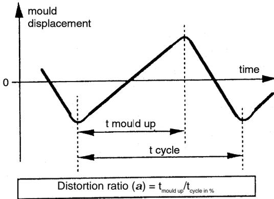
**Figure 7.** Triangular mode of oscillation (Darle *et al* 1993).
