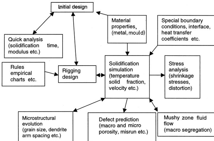
**Figure 4.** Typical architecture of a comprehensive solidification modelling system.
