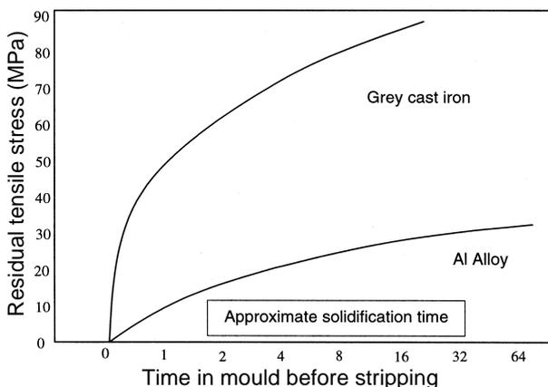
**Figure 2.** Residual stresses in aluminium alloy and grey iron castings as a function of stripping time.
