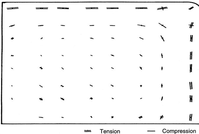
**Figure 11.** One quadrant of the principal stress field after four minutes.
