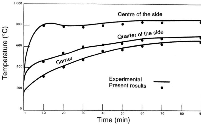
Figure 8. Temperature curve for inner wall of mould.
