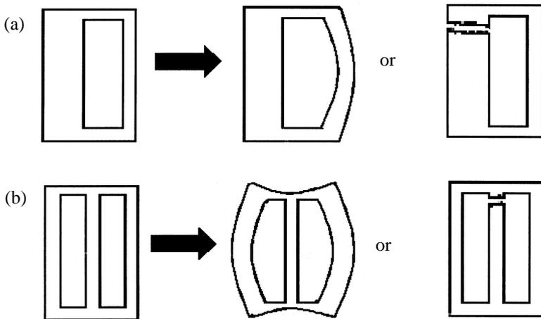
**Figure 1.** (a) A thick/thin section casting showing tensile stress in the thick section. (b) An even-walled casting showing internal tensile stresses.
