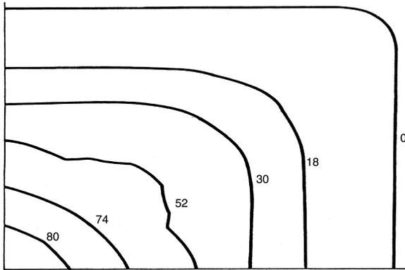
**Figure 10.** Solidification fronts for one quadrant of the ingot.
