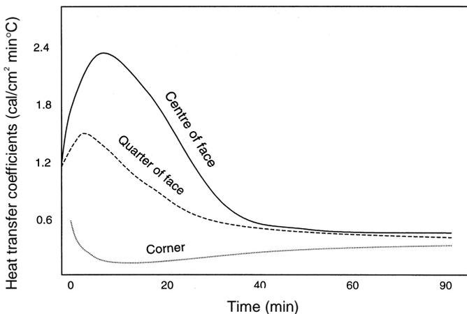
**Figure 7.** Average heat transfer coefficients in air gap.
