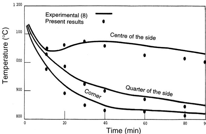
Figure 9. Average value of ingot surface temperature.
