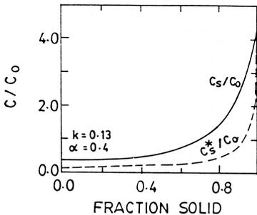
Figure 2. Calculated segregation of phosphorus in *d*-iron (Flemings 1990).
