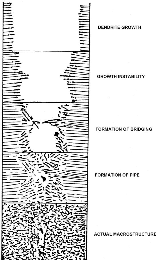
**Figure 12.** Formation of mini-ingot in continuous casting (Moore 1984).
