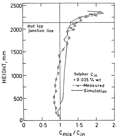
**Figure 8.** Comparison of measured and predicted macrosegregation variation of sulphur along the vertical centreline of the ingot (Gu & Beckermann 1999).
