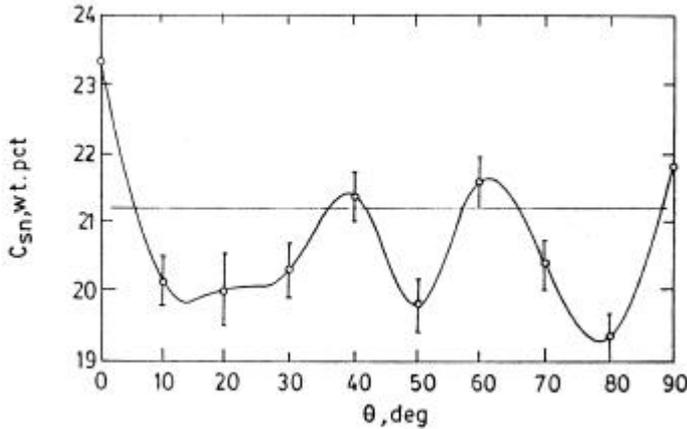
**Figure 7.** Circumferential variation of measured Sn concentration at  $r^* = 0.30$  and  $z^* = 0.83$  (Prescott & Incropera 1996).
