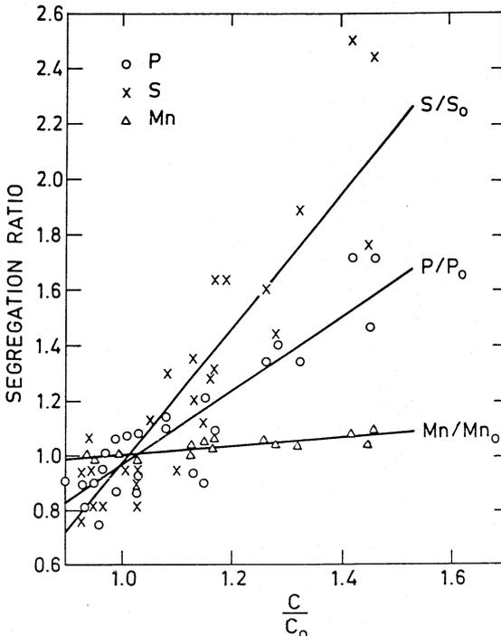
**Figure 13.** Relationship between segregation ratios of S, P and Mn with that of carbon in cast billets (Moore 1984).
