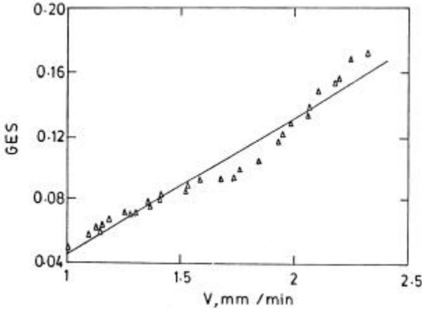
**Figure 9.** Global macrosegregation intensity of carbon as a function velocity of interdendritic liquid (Radovic *et al* 1999).
