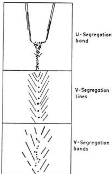
**Figure 14.** Some features of macrosegregation in longitudinal section of continuously cast billets (Goyal & Ghosh 1992).
