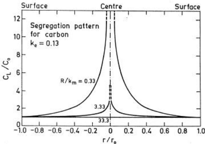
**Figure 10.** Transverse segregation profile for carbon in CC product calculated from Burton's equation (Ghosh 1990).
