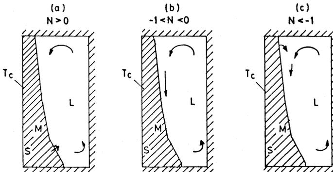
**Figure 5.** Thermosolutal convection pattern in the melt and mushy zone of a solidifying alloy: (a) solutal buoyancy forces augmenting thermal buoyancy force, (b) solutal buoyancy forces opposing thermal buoyancy forces, with thermal buoyancy dominating in the mushy zone, and (c) solutal buoyancy forces opposing and dominating thermal buoyancy forces in the mushy zone (Prescott & Incropera 1996).
