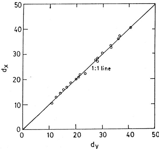
**Figure 15.** Comparison between measured and computed positions of CET boundary from the centre of billet samples with corrected pouring temperature (Choudhary & Ghosh 1994).
