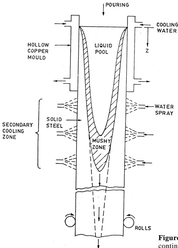
**Figure 11.** Ideal pool profile in continuous casting process (Ghosh 1990).
