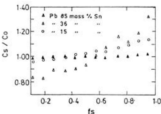
**Figure 6.** The longitudinal macrosegregation for Pb–Sn binary alloys upward directionally solidified under the conditions of  $R = 0.93$  cm/h and  $G = 36.5$  K/cm (Li *et al* 1999).
