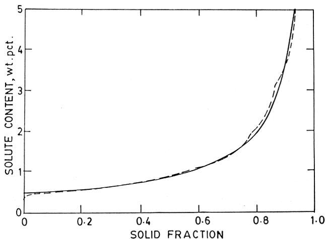
**Figure 3.** Distribution of solute as calculated with the Gulliver–Scheil model (full line) and cumulative distribution obtained from the experimental points (dashed line) (Lacaze & Lesoult 1999).
