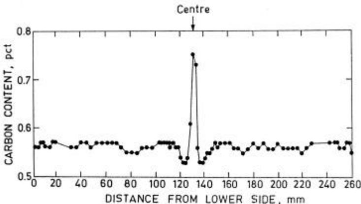
**Figure 1.** A typical concentration profile in an earlier continuous slab casting (Moore 1984).
