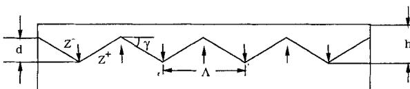
Figure 1. Triangular profile of the periodic domain inversion grating induced by titanium indiffusion in LiNbO<sub>3</sub>.  $h$  is the depth of the triangular grating.
