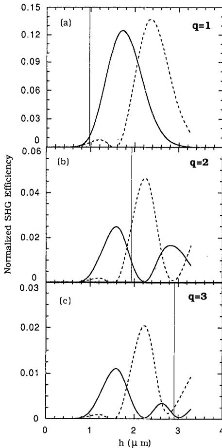
**Figure 3.** The SHG conversion efficiency (normalized to ideal laminar structure) as a function of domain inversion grating depth  $h$  for  $TM_{00}^{2\omega}$  (—) and  $TM_{10}^{2\omega}$  (----) modes in the case of (a) first-, (b) second-, and (c) third-order QPM SHG in the optimized APE  $LiNbO_3$  channel waveguides ( $\lambda^\omega = 865$  nm).
