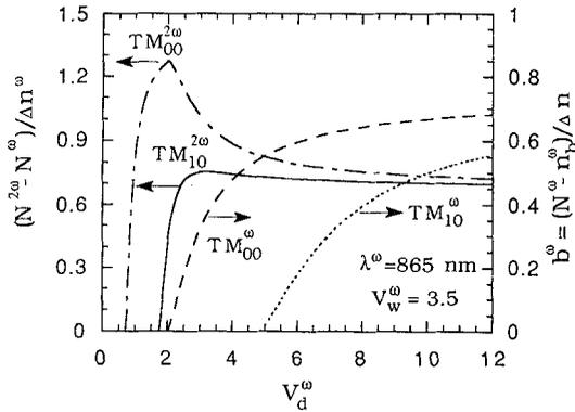
**Figure 2.** Normalized mode index mismatch between the fundamental ( $TM_{00}^{2\omega}$ ) and the harmonic ( $TM_{00}^{2\omega}$  and  $TM_{10}^{2\omega}$ ) modes and normalized mode indices for  $TM_{00}^{\omega}$  and  $TM_{10}^{\omega}$  modes in APE LiNbO<sub>3</sub> channel waveguides as a function of normalized waveguide depth  $V_d^{\omega}$  ( $\lambda^{\omega} = 865$  nm).
