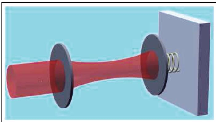
**Figure 4.** A typical cavity optomechanical system is driven by a laser. The left mirror is fixed while the right mirror is attached to the spring providing the mechanical mode in the system.
