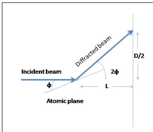
**Figure 2.** Electron diffraction in Thomson's experiment.
