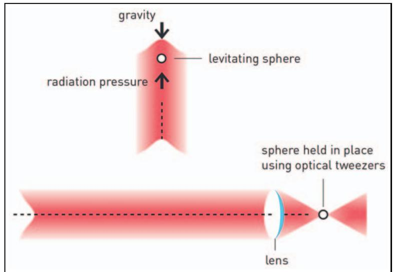
Ashkin reasoned and proved that the same light pressure that sweeps from a comet's tail could be used to push a micron-sized ball around in the lab. He demonstrated unequivocally that the forces at play within the laser beam drew a bead into the centre of the laser beam and trapped it there.
