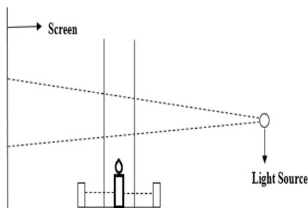
**Figure A.** Schematic of the shadowgraph experimental setup. The glass tube had a square cross-sectional area of  $25 \text{ cm}^2$  and a height of  $30 \text{ cm}$ . The light source creates a shadow of the hot and cold air currents on the translucent screen. The optical camera (Nikon Coolpix P7800) was behind the screen to record the shadow patterns.
