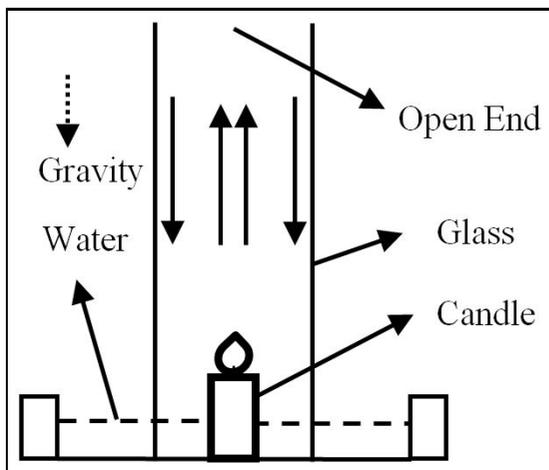
**Figure 1.** Schematic of the experimental setup. Candles used were 1 and 2.5 cm in diameter with 1 and 2 mm thick wicks, respectively. Diameter of the glass tube was 58.6 mm and their heights used were 24, 30, 38, 43.5, 48, 55.5, and 60 cm.
