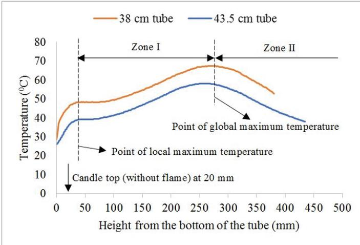
**Figure 5.** Tube outer surface temperature vs. height from tube bottom during steady state. Two maxima are observed in surface temperature – a local one near the flame and a global one at about 275 mm.
