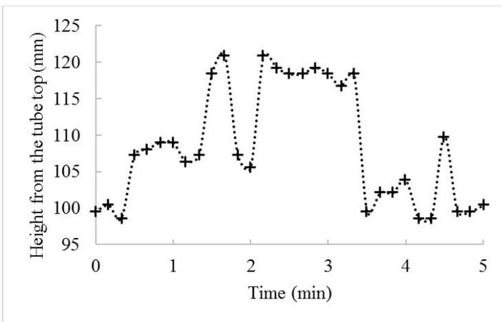
**Figure 6.** Variation of the point of maximum temperature with time (38 cm tube height, tube diameter 58.6 mm and 2.5 cm diameter candle). Note that the variations in position of the temperature maxima are approximately equal to the flame height.
