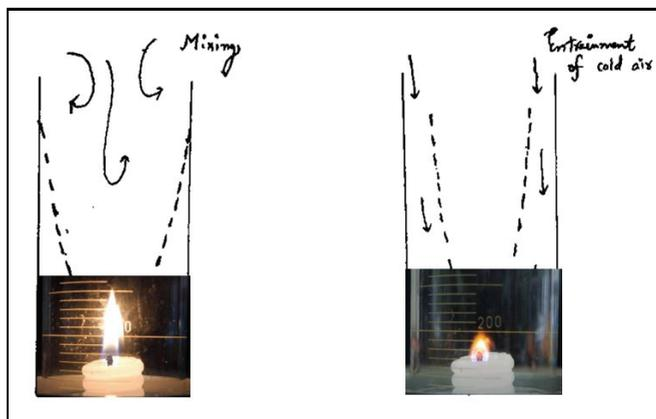
**Figure 4.** Thermal images of tubes with two different heights but the same glass tube diameter (58.6 mm) and the candle diameter (2.5 cm).
