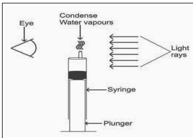
**Figure 3.** Setup for observing condensed water vapour.
