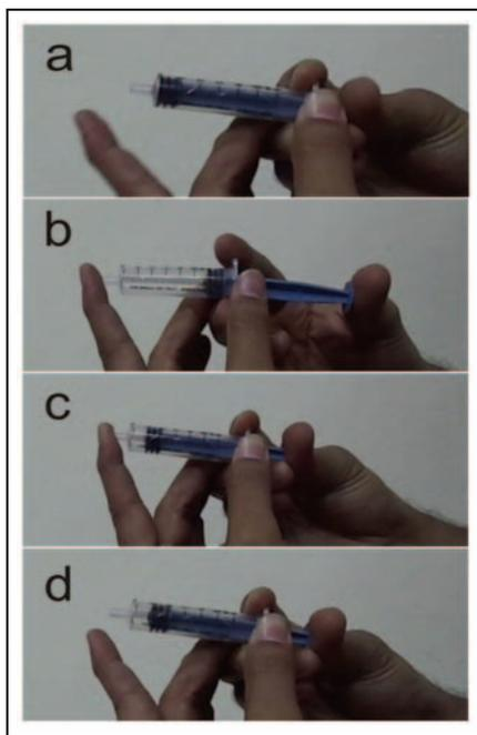
As shown in *Figure 4d*, the instant the index finger is removed, the condensed vapour inside the 1 ml volume is completely expelled outside by the pushing of the plunger until its volume inside the syringe is zero.
