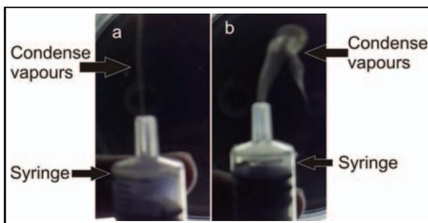
as an ‘isothermal compression’. Hence, no cognizable heating effects are observed in this process. At the minimum volume when the air is fully compressed, we can estimate the final temperature and pressure using the equation for adiabatic compression as given in *Box 3*.
