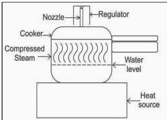
the steam pushes the regulator against the gravity and the vent pipe opens. At the same instant, the accumulated steam from inside the cooker escapes through the vent pipe into the atmosphere while making the whistling sound.
