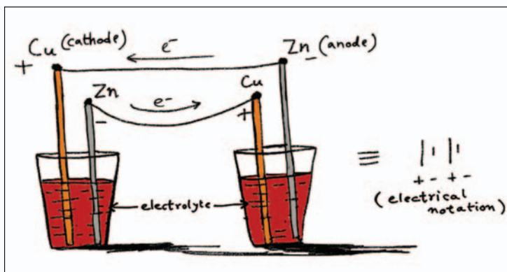
Then, connect a zinc rod of one glass to a copper rod of the other glass using electric wires (see *Figure 4*). Thus, the other free rods become free electrodes of a battery. If a voltmeter ( $V$ ) is connected to the electrodes you will see a finite voltage reading. You can repeat the same steps by inserting the metal electrodes into various fruits or vegetables and compare.
