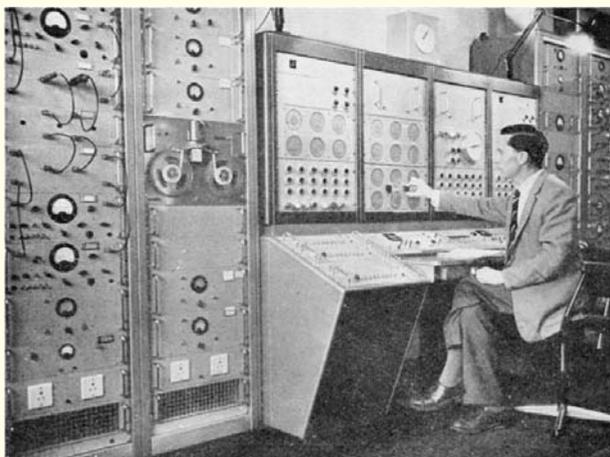
Fig. 3. The control desk and part of the receiving system
