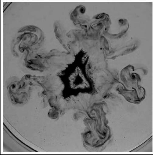
**Figure 2.** Pattern formed by a drop of isopropanol-oleic acid mixture (with dye) spreading on a pool of water.
