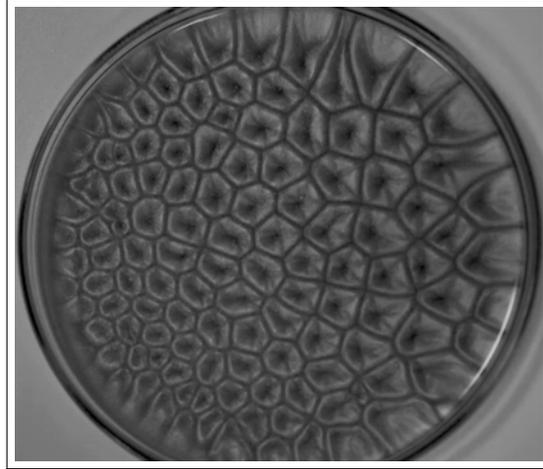
For sustained Marangoni convection, the induced motion at the surface must be stabilised by viscous drag and thermal diffusion.
