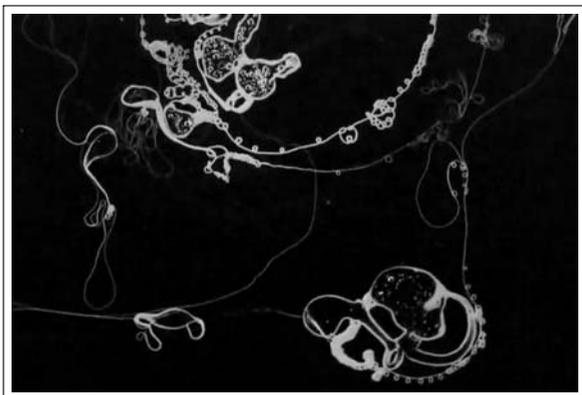
**Figure 5.** Filamentary structures formed by drops of liquid Duco cement spreading on a pool of water.
