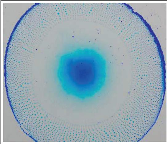
**Figure 3.** Pattern formed by drops of aqueous isopropanol (with dye) spreading on a pool of sunflower oil.
