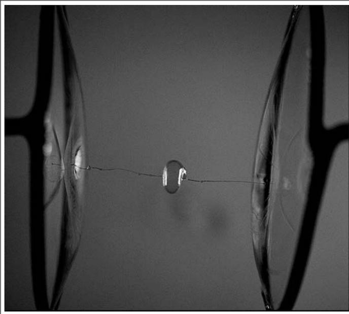
**Figure 4.** A soap bubble linked by filaments to planar discs, during the breakup of a catenoidal bridge.
