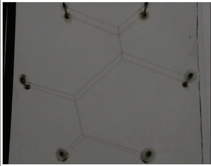
**Figure 5.** An analog solution to the motorway problem for a regular hexagonal configuration (see the text for discussion).
