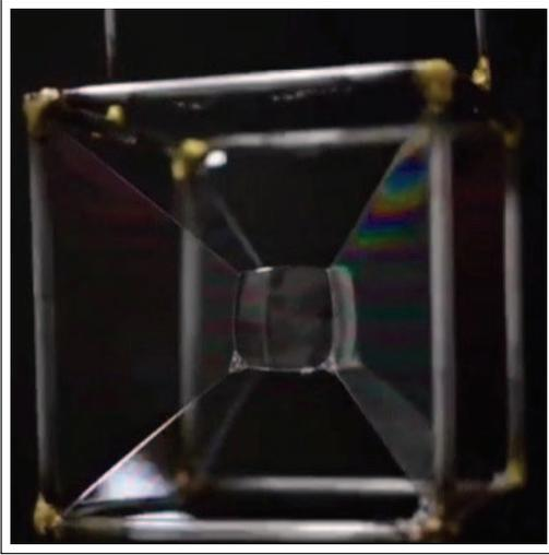
**Figure 2.** An air bubble trapped within a soap film in a cubical frame.
