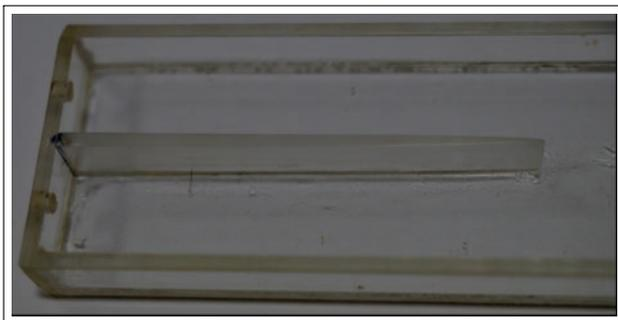
**Figure 4.** Plexiglass rectangular channel with splitter plate and two inlet holes.
