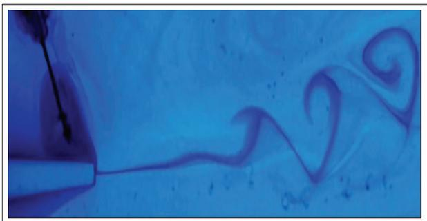
**Figure 5.** Kelvin-Helmholtz vortices in a rectangular channel at the interface of two parallel streams of aqueous corn-syrup.
