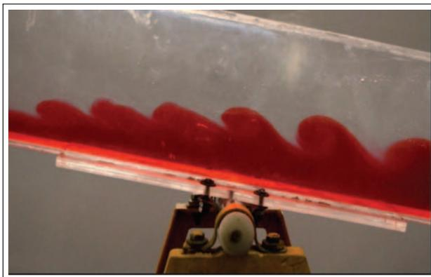
for a few seconds, approximately seven vortices may be seen at the interface (see *Figure 3*). The flow undergoes a transition to turbulence and rapid mixing ensues at the interface.
