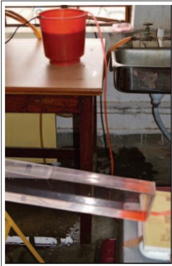
**Figure 2.** Filling the plexiglass cell with dyed brine *via* a submersible pump placed inside the bucket.
