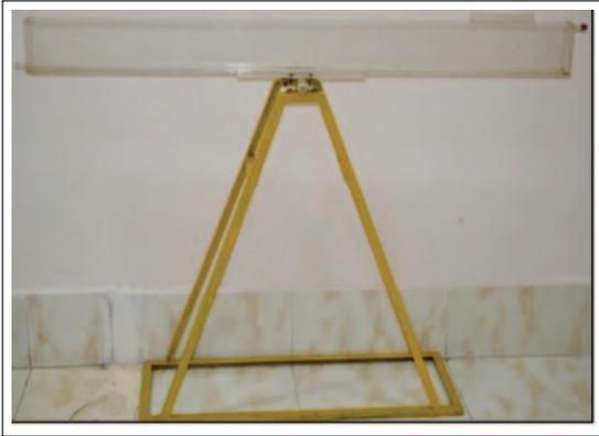
**Figure 1.** Experimental setup for demonstrating Kelvin–Helmholtz instability.
