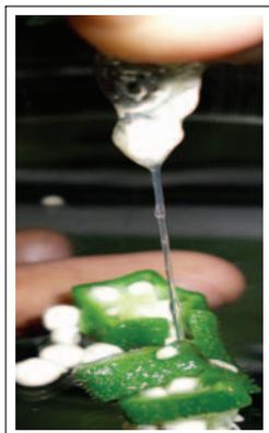
**Figure 1.** Formation of an elastic filament using okra mucilage.
