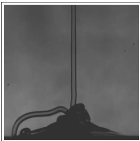
**Figure 3.** A stream of liquid detergent bouncing off a heap of the same liquid as a demonstration of the Kaye effect, imaged using a high-speed camera.
