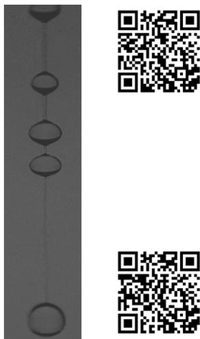
**Figure 4.** A jet of 100 ppm aqueous polyacrylamide solution, imaged using a high-speed camera.
