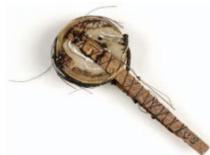
**Figure 4.** The world’s first superconducting magnet, consisting of a wire coil made of lead, was manufactured in the Leiden (The Netherlands) Physics Laboratory in 1912. Reprinted with permission from [6].
