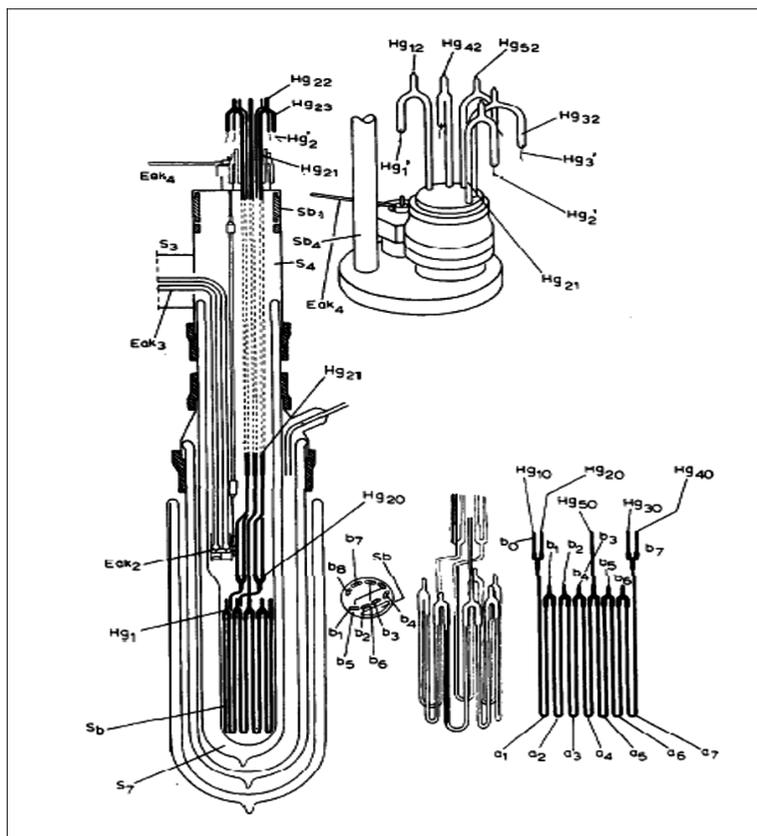
**Figure 1.** Bottom part of the cryostat in which resistance of Hg was determined. Reprinted with permission from [2] © The Nobel Foundation (1913).
