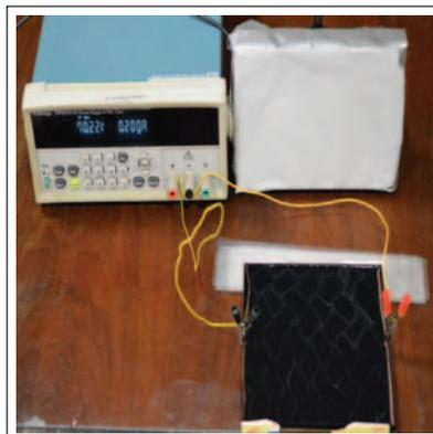
**Figure 3.** Base state of Kolmogorov flow at a DC current = 0.05 A.
