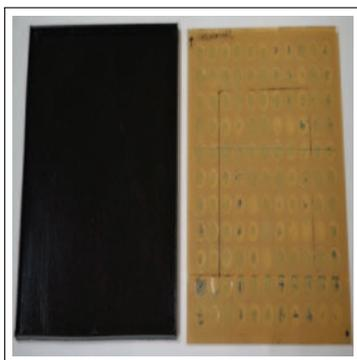
**Figure 1.** Black plexiglas tray (left) and plexiglas perforated sheet (right) with an  $11 \times 11$  array of neodymium alloy disk magnets.
