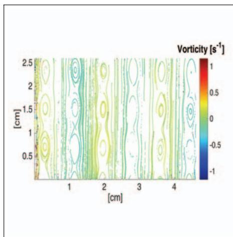
**Figure 6.** Scatter plot of the magnitude of vorticity at a DC current = 0.1 A.
