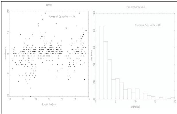
**Figure 7.** Time observations with the temporary markings made on the Samrat Yantra quadrant and floor. Markings were made for every minute and public observations were conducted on winter solstice day 2006. The figure on the left shows the time measurement errors, and the one on the right shows the error frequency distribution.
