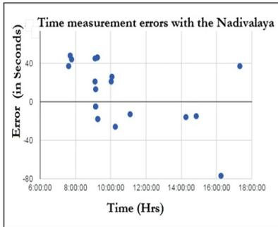
**Figure 5.** Errors in time measurement taken with a small Nadivalaya at the Jantar Mantar observatory on the Manmandir terrace, Varanasi.
