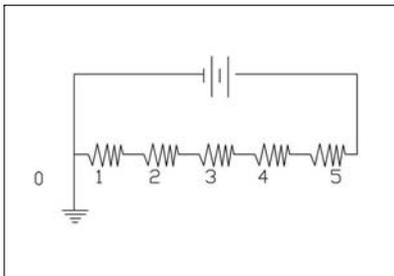
**Figure 13.** An electrical circuit for the solution of the drunkard's walk problem.
