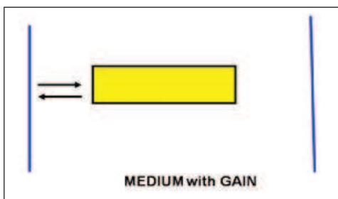
Fabry–Perot Resonator formed by two plane parallel mirrors (*Figure 1*). Let us see how this can be used to control light emission from the laser.
