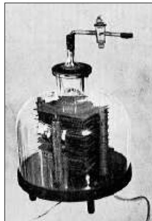
**Figure 1.** Ionization chamber built by Shyamadas Chatterjee for detection of spontaneous fission of uranium.
