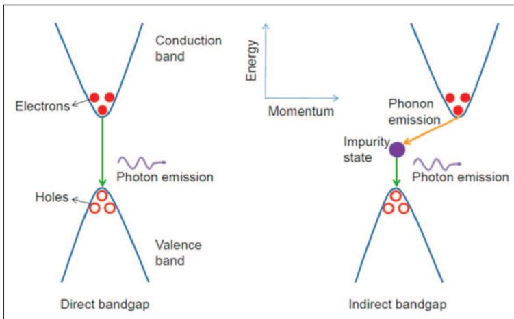
**Figure 4.** Schematic of radiative recombination in direct and indirect bandgap semiconductors. An impurity energy state is needed to facilitate recombination in indirect bandgap materials [29].
