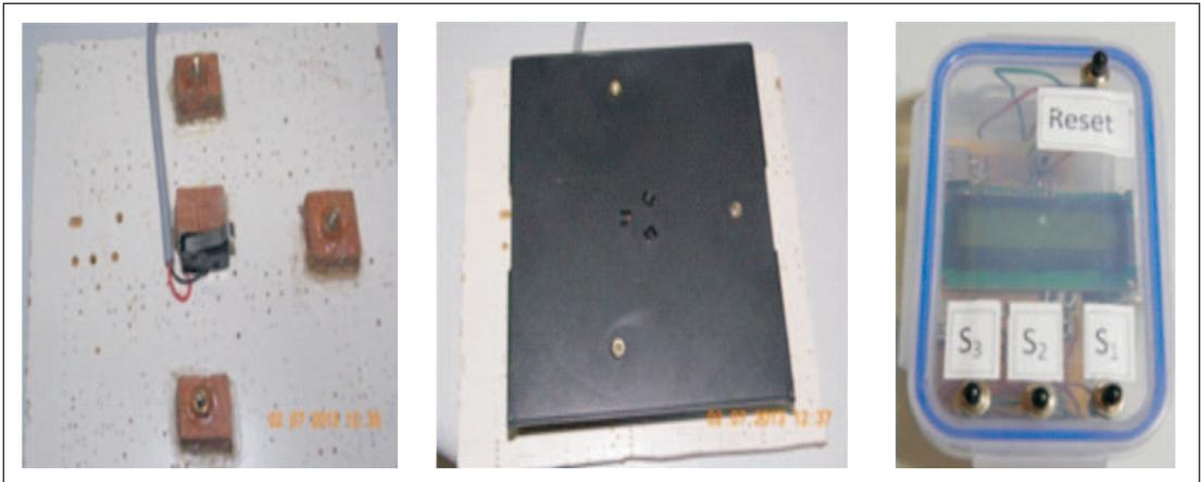
velocity of launch and time of flight can be determined. Once reading is taken, the reset switch is pressed for taking the next reading. The photogates (attached to launcher and the contact sensor pad) are connected to the microcontroller through USB ports. The timer can also be used in simple pendulum and free fall experiments. In this article, only the projectile motion experiment is discussed.
