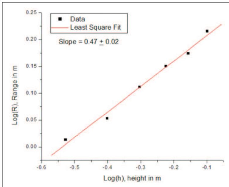
the value of the slope equal to  $0.47 \pm 0.02$ . This suggests that the value of  $n$  is 0.5 and hence,  $R \propto \sqrt{h}$ .
