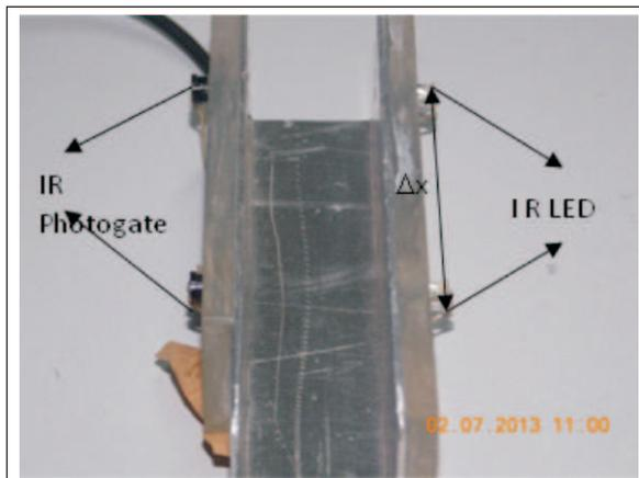
can be measured by noting the time duration ( $\Delta t$ ) between the two triggering. The speed of the projectile is  $\Delta x/\Delta t$ . The entire unit is fixed in the front portion of the projectile launcher such that the projectile passes through the photogate and hence its speed could be recorded for every launch.
