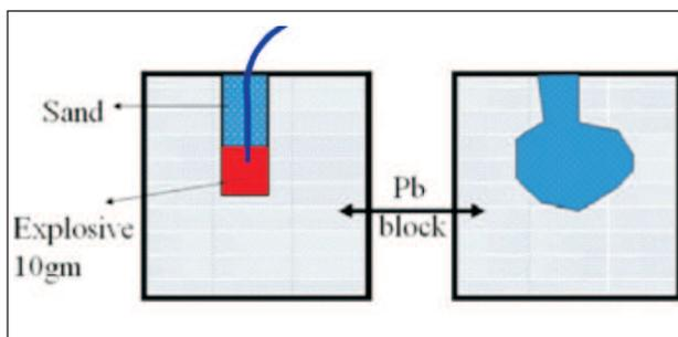
**Figure 1.** The lead block test.
