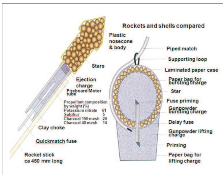
**Figure 4.** Comparison of a single-colour skyrocket and shell [1].
