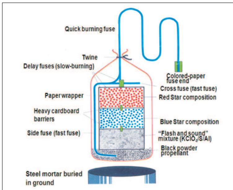
**Figure 5.** Schematic diagram of a multi-colour rocket [2].
