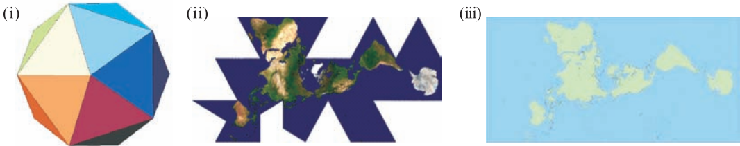
Figure B. (i) An icosahedron with 20 faces, (ii) the surface of the Earth projected onto an icosahedron and developed in a particular way, (iii) Dymaxion projection of the Earth where the entire world looks like an island in a great ocean.
