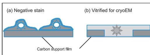
**Figure 5.** Macromolecular protein complexes specimen (a) negatively stained complex with high contrast lying on continuous carbon film (b) complex lying in a vitrified ice on a holey carbon grid with low contrast. The complex is suspended in a vitrified ice (hole) thus preserving the solution state.
