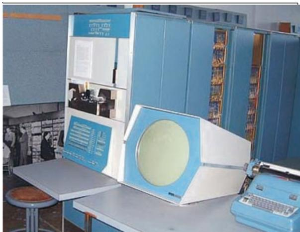
**Figure 1.** The console of PDP-1 computer. See the large CRT display and an IBM Selectric typewriter for interactive use of the computer. Courtesy: Image reproduced with permission from <http://ed-thelen.org/comp-hist/vs-dec-ddp-1.jpg>
