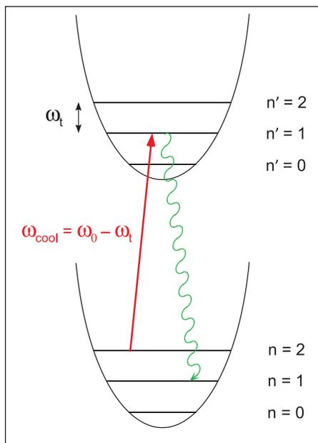
**Figure 2.** Principle of sideband cooling. The motional degrees of freedom in the trap are quantized to form a set of evenly spaced levels separated by  $\omega_t$ . The cooling laser is tuned to the lower motional sideband, i.e., at  $\omega_0 - \omega_t$ , so that the ion loses one quantum of vibrational energy in each absorption–emission cycle.
