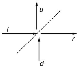
**Figure A.** Illustrating the S-matrix of a half-silvered mirror, which transforms two incident amplitudes  $l$  and  $d$  into two outgoing amplitudes  $u$  and  $r$ .
