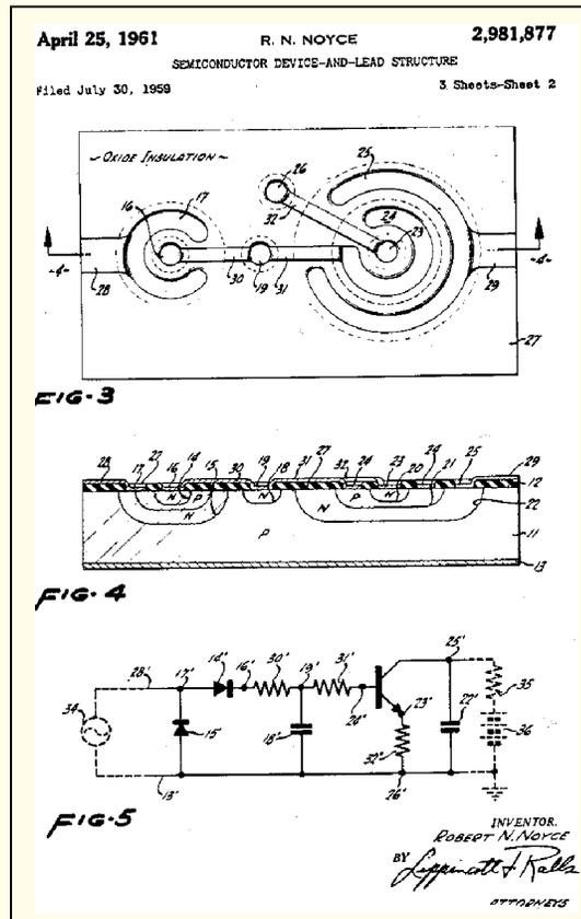
Fig. 6. Noyce patent 2,981,877 showing planar structure with evaporated aluminum interconnections adherent to the surface.
