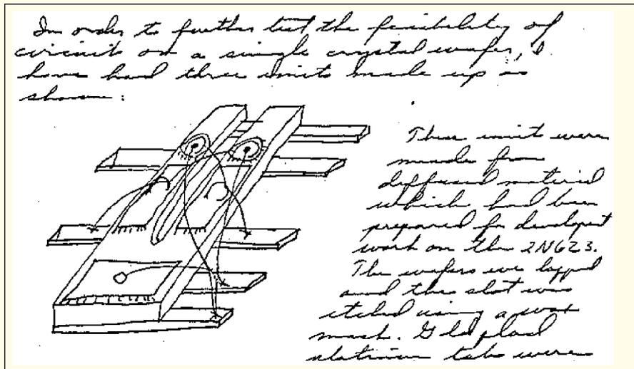
**Fig. 3.** Page of Kilby engineering notebook describing a flip-flop built from an existing diffused germanium wafer.
