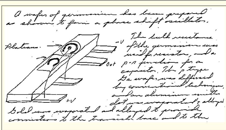
**Fig. 2.** Page of Kilby engineering notebook describing a phase shift oscillator built from an existing diffused germanium wafer.
