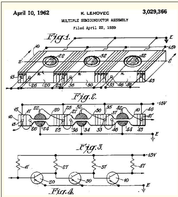
Fig. 5. US Patent 3,029,366, describing Lehovec's alternating p-n junctions for isolation.
