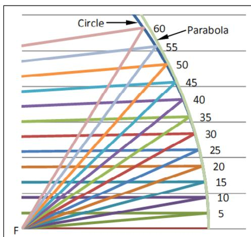
**Figure 6.** Reflection of rays emanating from the focus F and incident upon a spherically concave mirror at different angles with the principal axis as indicated alongside the ray. The parabola profile is shown for comparison.
