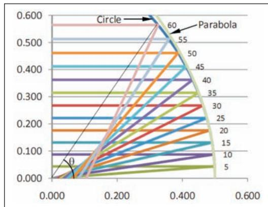
**Figure 8.** Reflection of rays incident upon a spherically concave mirror parallel to the principal axis. The numbers 5, 10, ..., 55, 60 indicate the values of  $\theta$  for the rays next to which they are written.
