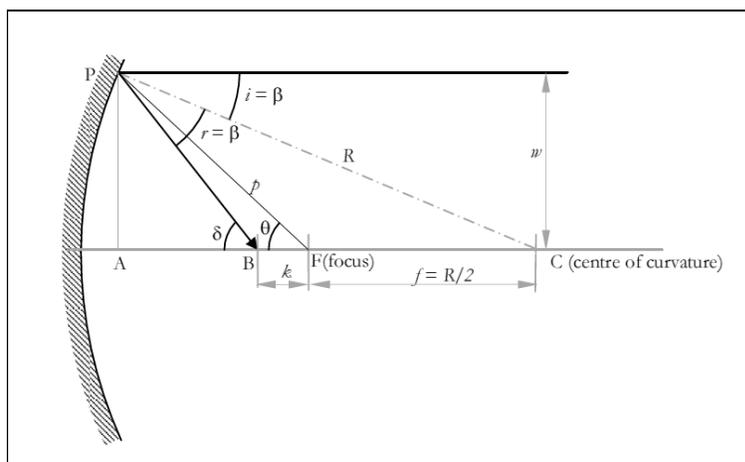
**Figure 7.** Behaviour of a ray incident parallel to the principal axis and at a distance from it.
