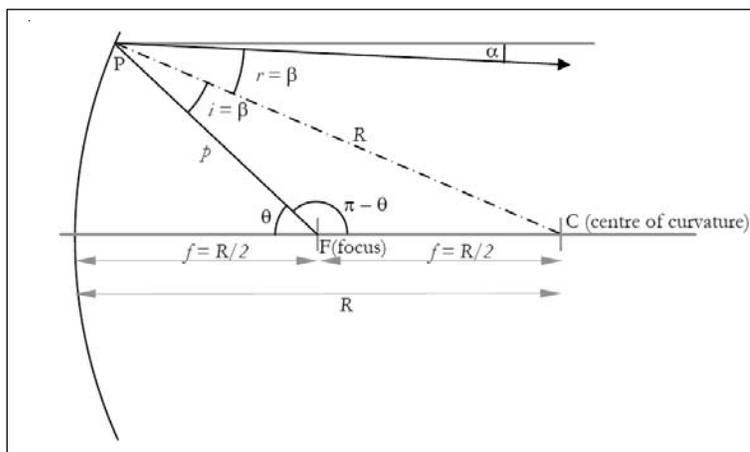
**Figure 3.** Geometry of ray reflection through a point away from the principal axis.
