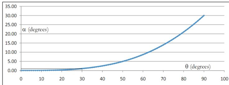
**Figure 5.** Deviation of reflected ray from axial direction.
