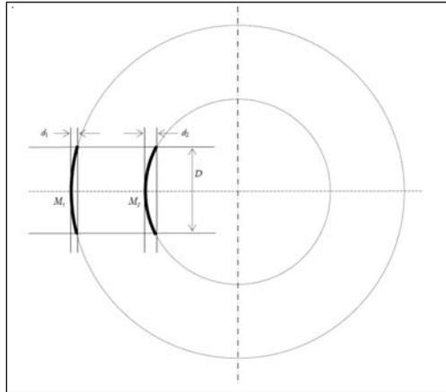
**Figure 12.** Given two spherical mirrors of the same rim diameter  $D$ , the one ( $M_1$ ) with the smaller depth ( $d_1$ ) can produce a parallel reflected beam better than the one ( $M_2$ ) with the larger depth ( $d_2$ ).
