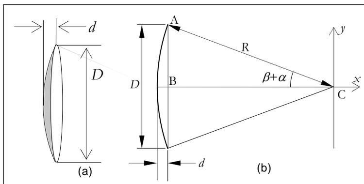
**Figure 10.** (a) The physically measurable parameters, depth  $d$  and rim diameter  $D$ , of a concave mirror. (b) The relationship between  $d$ ,  $D$ , and the radius of curvature  $R$  of the mirror.
