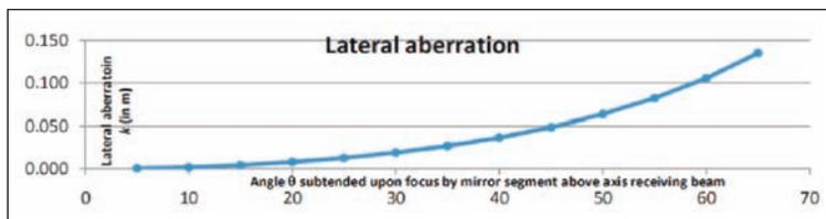
**Figure 9.** The amount by which a beam misses the focus as a function of its width; this is measured as the angle that half the mirror segment upon which it is incident subtends upon the focus.
