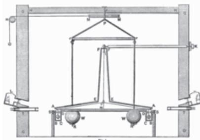
**Figure A.** Cavendish's torsion balance instrument.
