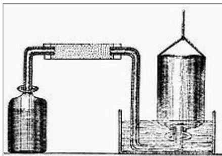
**Figure 4.** Cavendish's apparatus for making and collecting hydrogen.
