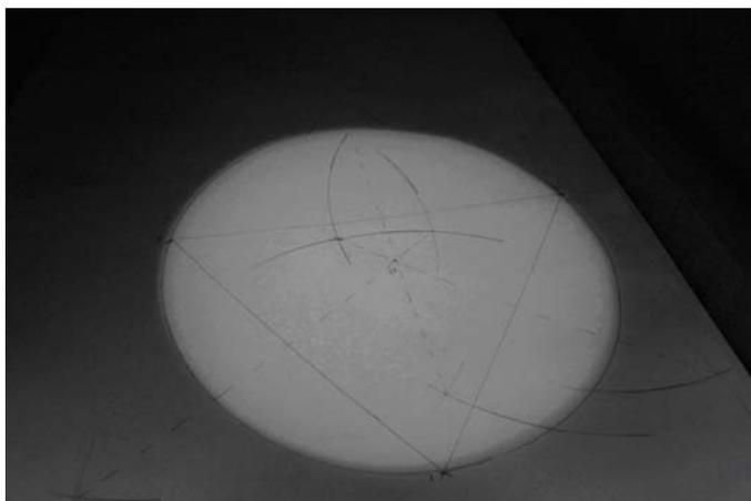
image of the Sun (rapidly, in order to avoid errors creeping in from the diurnal movement), drawing a triangle through these points, and then drawing the circumcircle of this triangle. The drawn circle should be placed in the projection box pointed towards the Sun, and errors in the determination of the diameter of the projected image of the Sun corrected iteratively.
